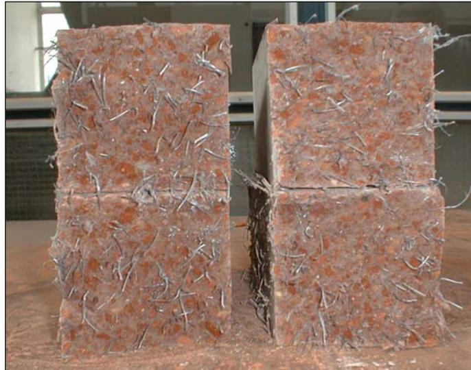
Figure 2: Specimens with recycled masonry aggregate
