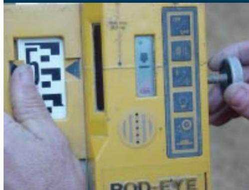
4. When the pointer on the staff is level with the laser-sending signal, the arrows will disappear, leaving a straight line.
