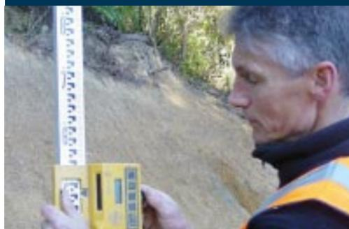
3. The final adjustment is done either by adjusting the receiver until the beeps become continuous, or by visually following the instruction given by either an up or down arrow.
