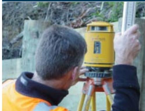
1. The laser instrument is set on the tripod then levelled by the centralising of bubbles at its base.
