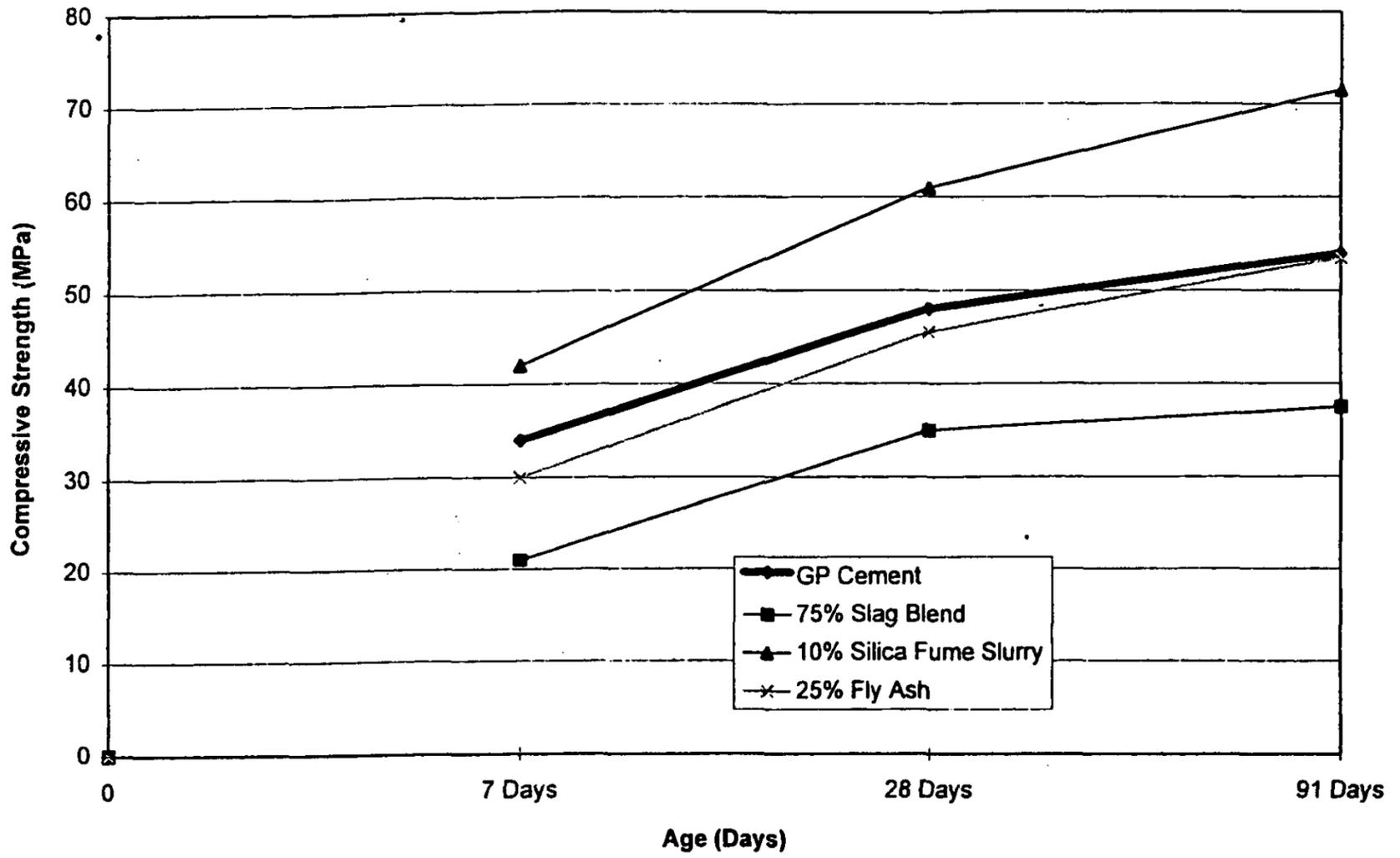
Fig. 2a—Compressive strength development for 325 kg cementitious mixes
