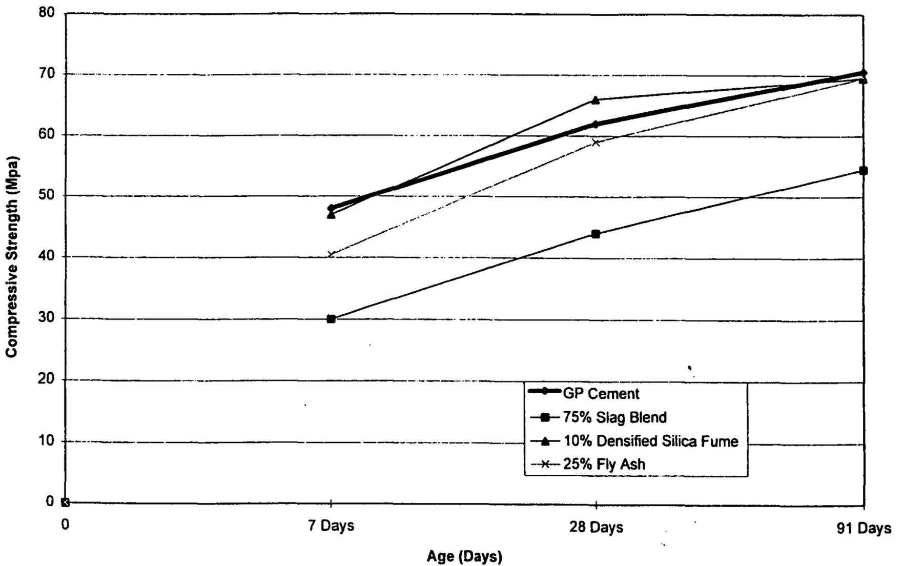
Fig. 2b—Compressive strength development for 440 kg cementitious mixes
