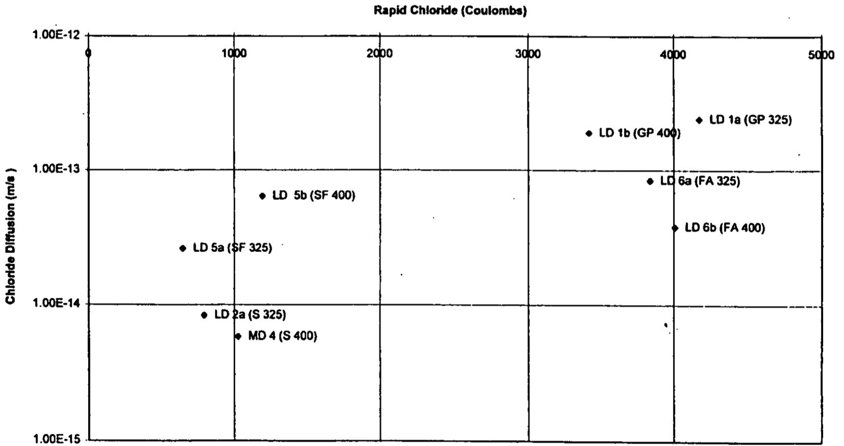
Fig. 4—Chloride diffusion verses rapid chloride test results
