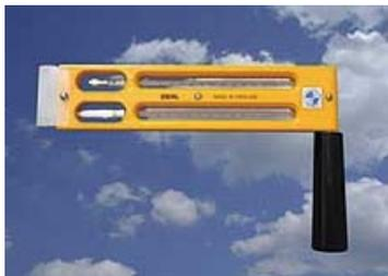
**Figure 1: Whirling Hygrometer**
