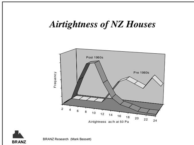
**Figure 7: Airtightness of New Zealand Houses**
