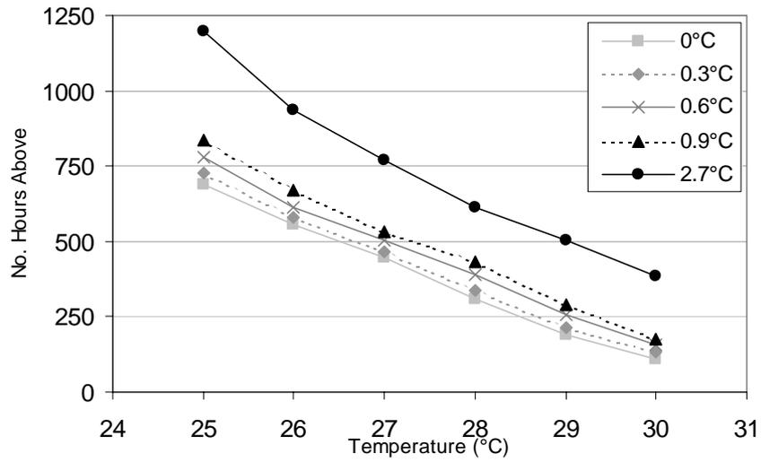
**Figure 2. Number of hours above temperatures with rising temperatures, naturally ventilated buildings, Auckland.**
