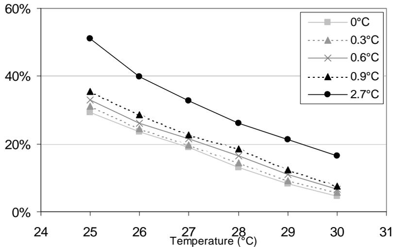
**Figure 4. Percentage hours above set temperatures, naturally ventilated buildings, Auckland.**
