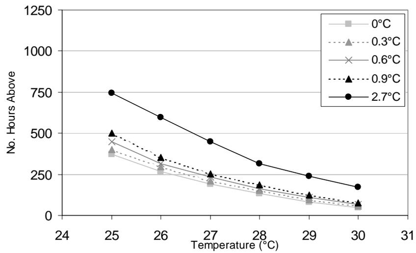
**Figure 3. Number of hours above set temperatures with rising temperatures, naturally ventilated buildings, Christchurch.**
