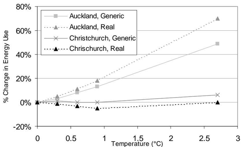
**Figure 1. Change in energy use for simulated buildings.**
