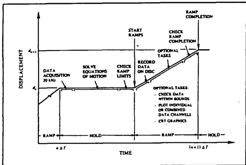
Figure 5. Tasks performed in each step of a pseudo-dynamic test (Mahin and Shing 1985).
