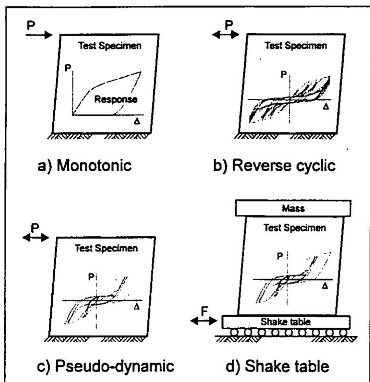
Figure 1. Specimen test methods
