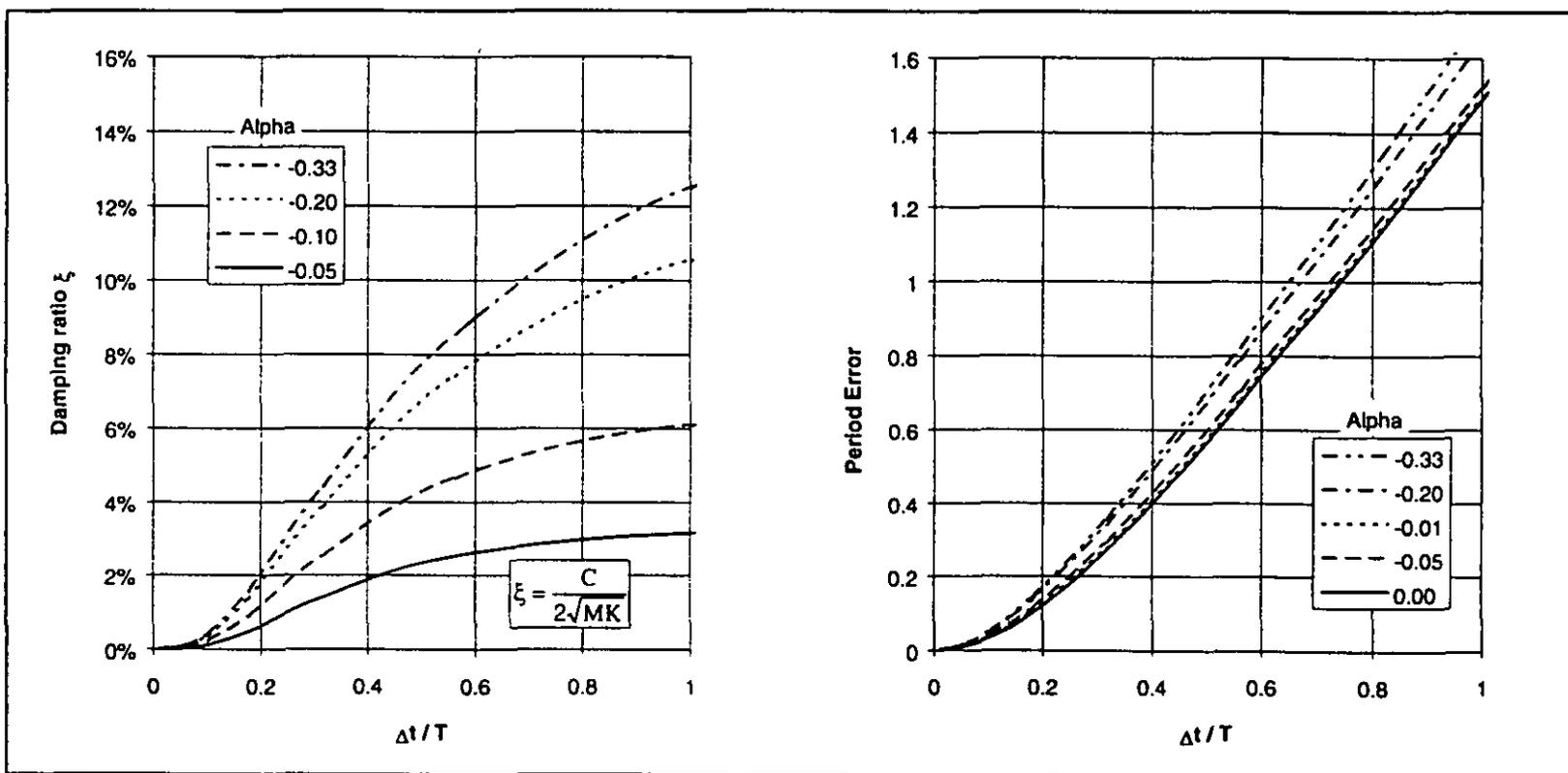
Figure 4. Damping and period error as a function of time step, natural period and  $\alpha$  (Hilber et al. 1977).
