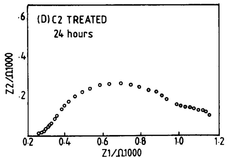
FIGURE 3 — Impedance diagrams for iron potentiostated at the corrosion potential and in contact with transverse section water-saturated wood in air. The equivalent circuit parameters are:
