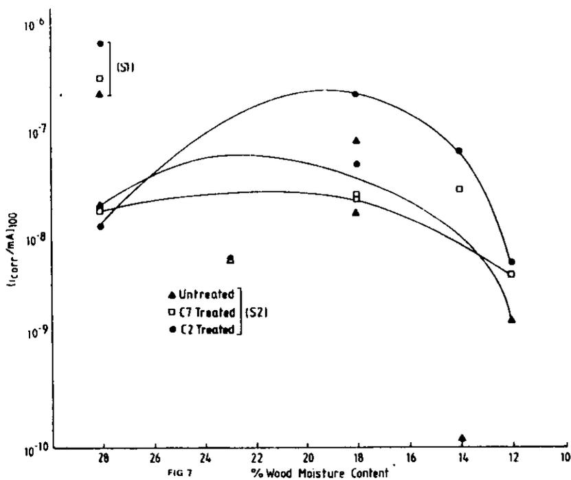
FIGURE 7 — Corrosion current vs wood moisture content for iron in contact with untreated and C2- and C7-treated wood after 100-day exposure. S1 and S2 refer to Samples 1 and 2 wood, respectively.
