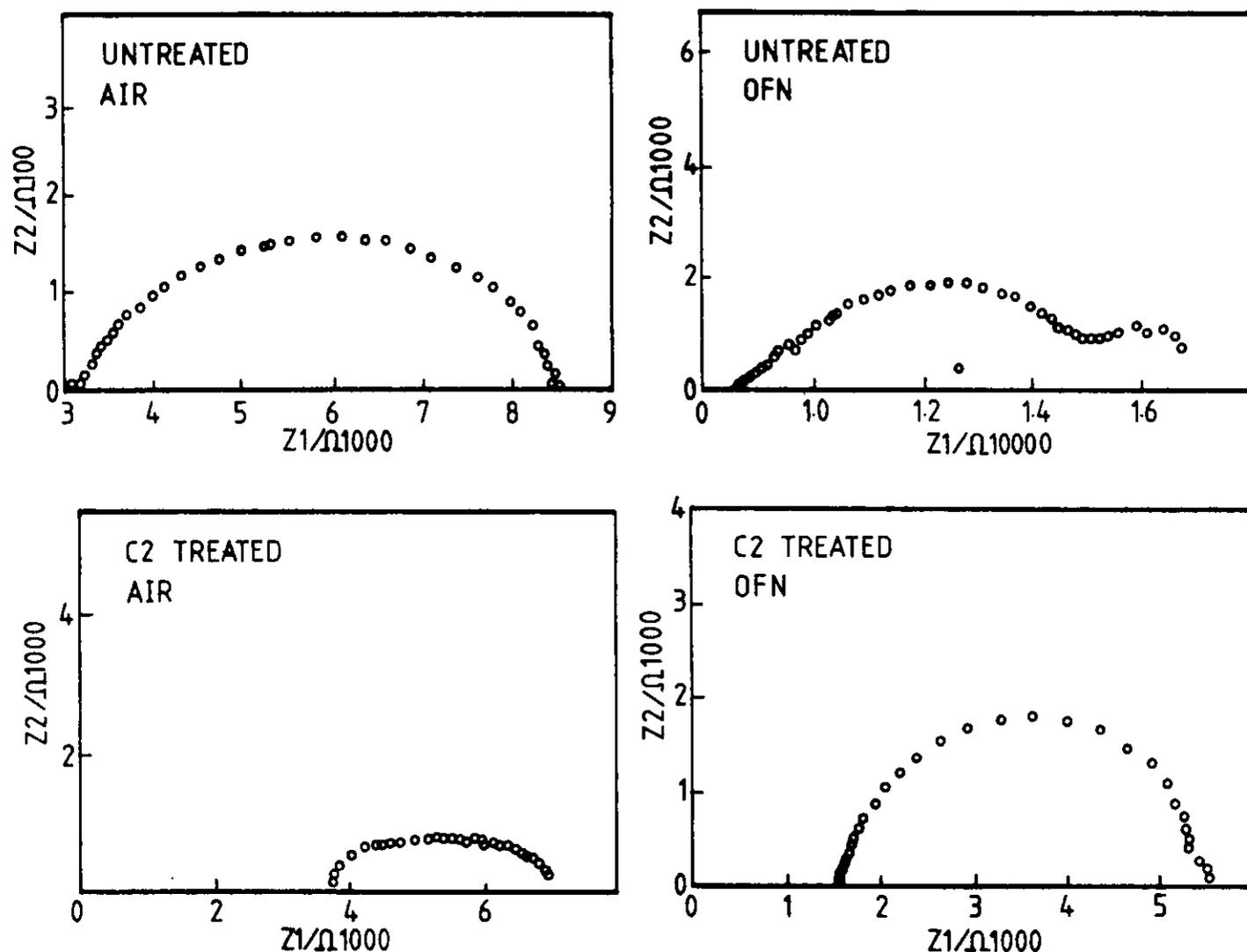
FIGURE 5 — Impedance diagrams for iron potentiostated at the corrosion potential in contact with water-saturated radial longitudinal wood in air and OFN. The electrode area = 0.25 cm<sup>2</sup>.
