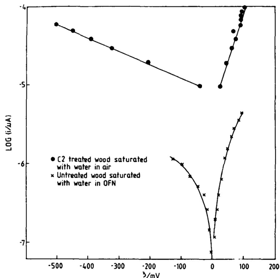
FIGURE 2 —  $\log i$  vs overpotential for iron in contact with water-saturated wood.
