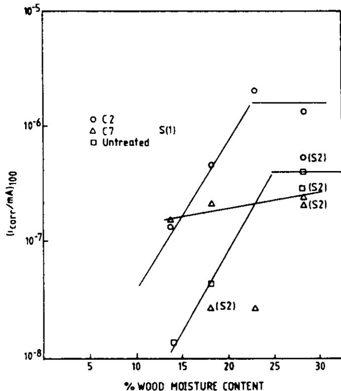
FIGURE 8 — Corrosion current vs wood moisture content for zinc in contact with untreated and C2- and C7-treated wood. S1 and S2 refer to Samples 1 and 2 wood, respectively.
