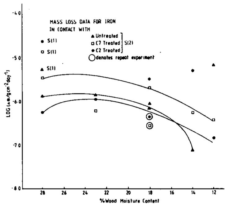
FIGURE 9 — Mass loss vs wood moisture content for iron in contact with untreated wood and C2- and C7-treated wood for Sample 2. S1 refers to Sample 1 wood.
