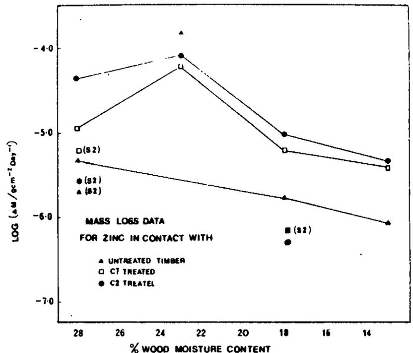
FIGURE 10 — Mass loss vs wood moisture content for zinc in contact with untreated wood and C2- and C7-treated wood from Sample 1. S2 refers to Sample 2 wood.
