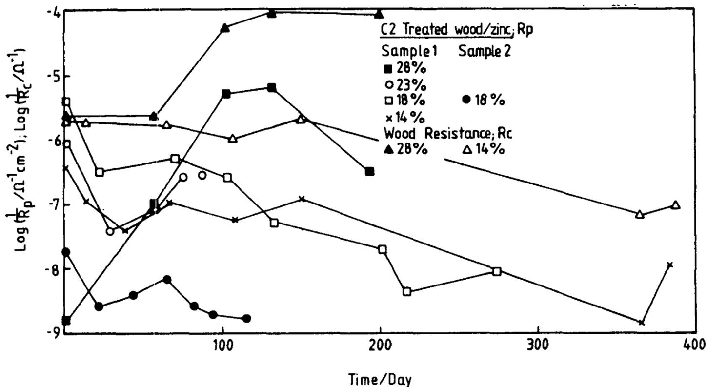
FIGURE 6 —  $\text{Log } R_p^{-1}$  ( $R_p$  = polarization resistance) and  $\text{log } R_c^{-1}$  ( $R_c$  = cell resistance) vs time for zinc in contact with C2-treated wood of different moisture levels.
