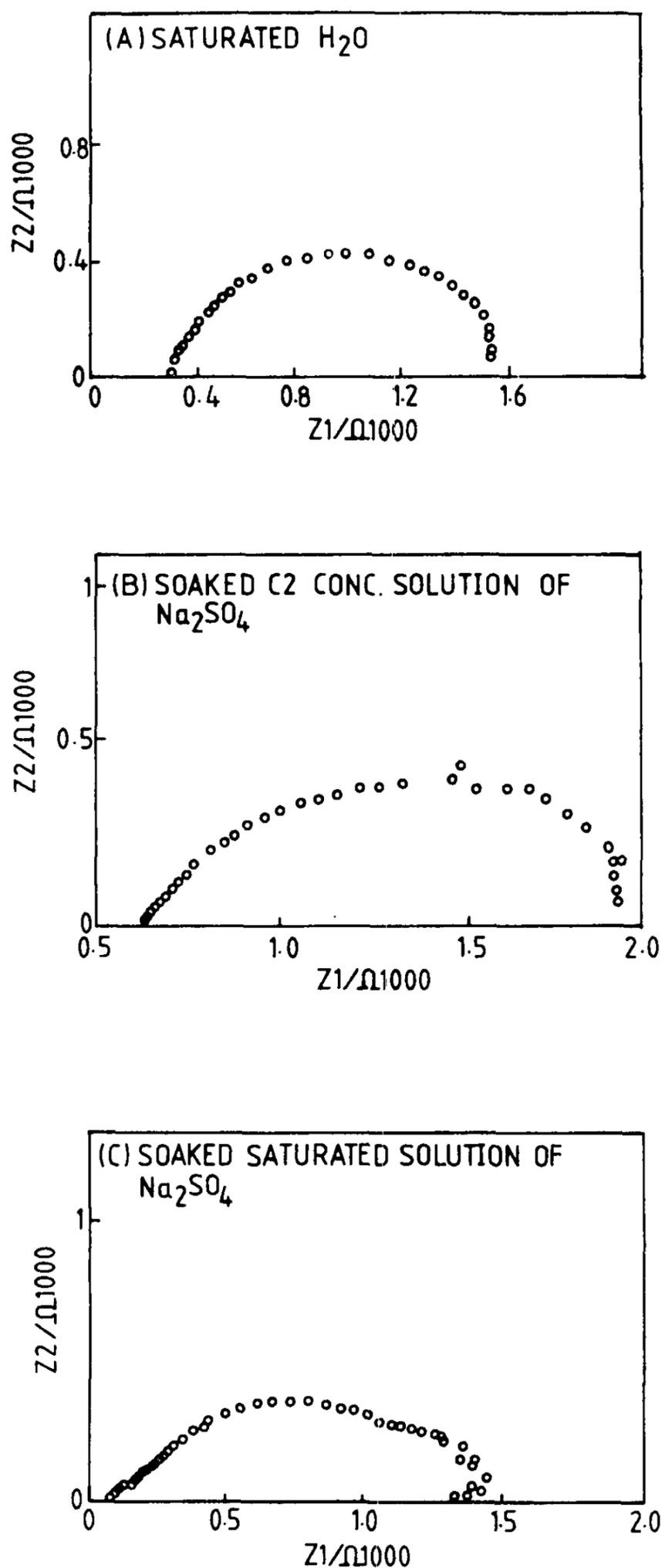
FIGURE 4 — Impedance diagrams for iron potentiostated at the corrosion potential in contact with transverse section water-saturated wood. The electrode area = 0.25 cm<sup>2</sup>. The wood is untreated and, before cell assembly, was soaked in (a) H<sub>2</sub>O, (b) Na<sub>2</sub>SO<sub>4</sub> solution of the concentration expected to be found in C2-treated wood (i.e., ~0.1 mol dm<sup>-3</sup>), and (c) in saturated Na<sub>2</sub>SO<sub>4</sub> solution.
