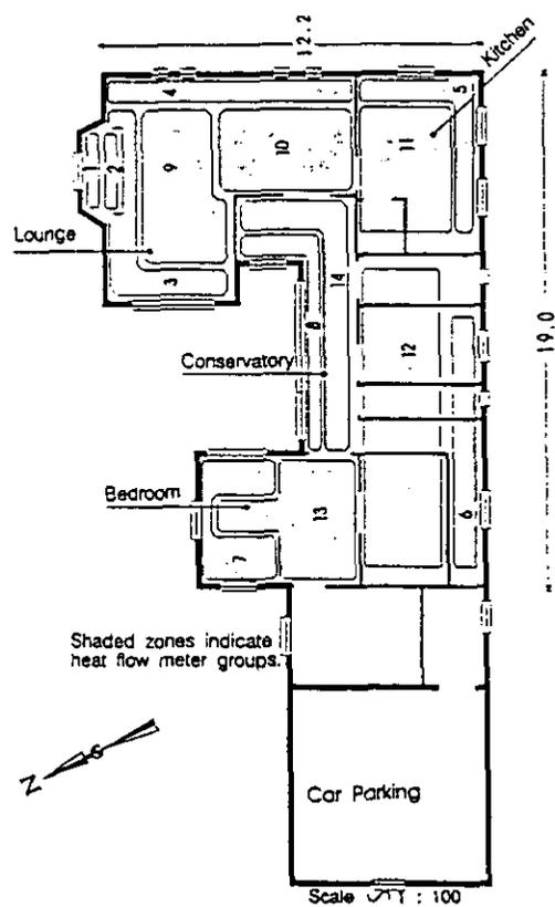
Figure 1 Floor Plan and Heat Metering Zones
