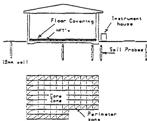
Figure 2 General Instrumentation Plan
