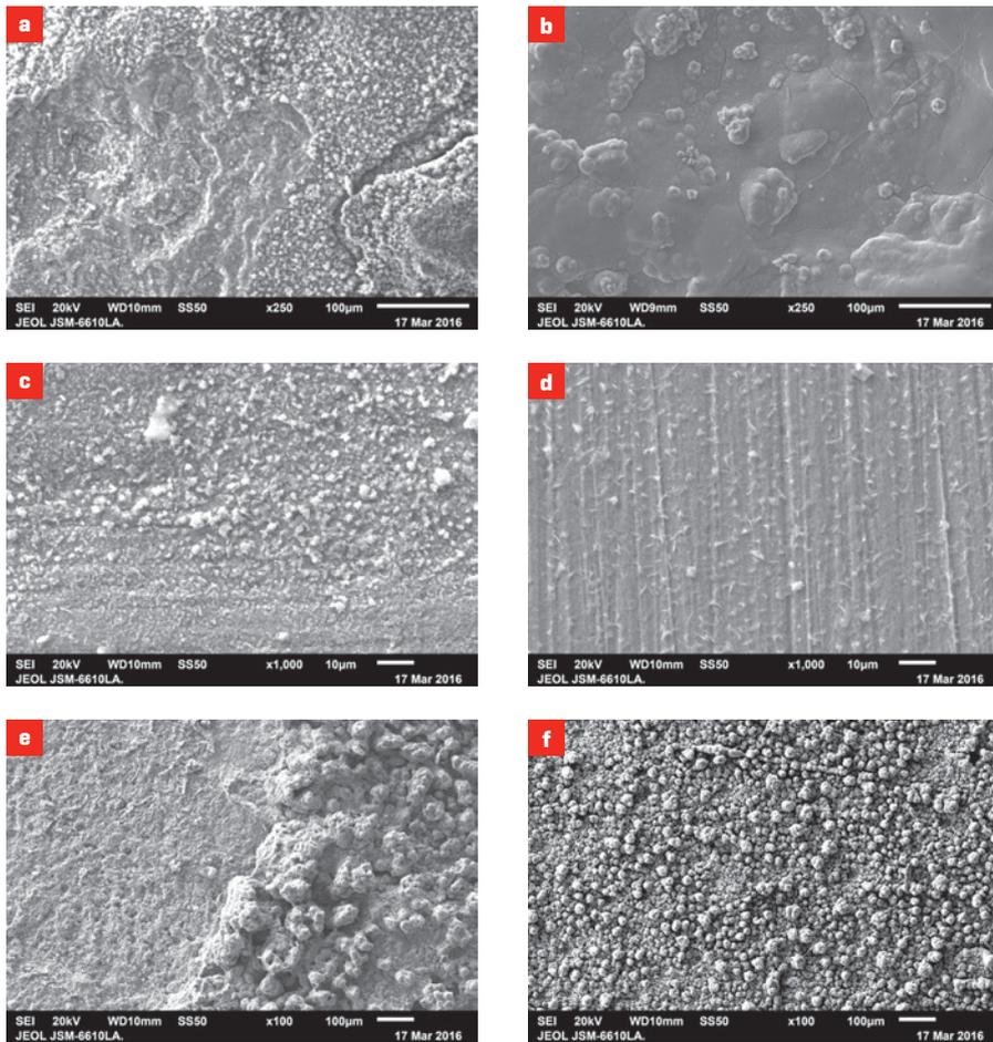
a) Mild steel at 5 m from a fumarole. b) Mild steel at 50 m. c) Zinc at 5 m. d) Zinc at 50 m. e) Copper at 5 m. f) Copper at 50 m.
