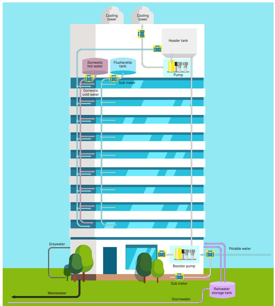
A simple schematic diagram of a rainwater harvesting system in a commercial building.
