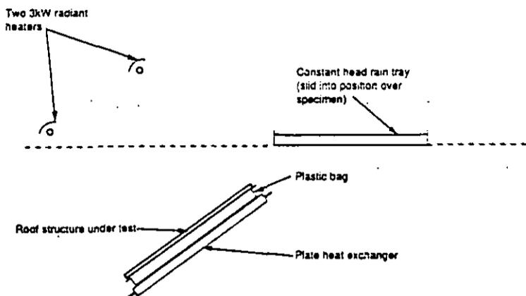
Figure 1 Schematic diagram of the test rig used
