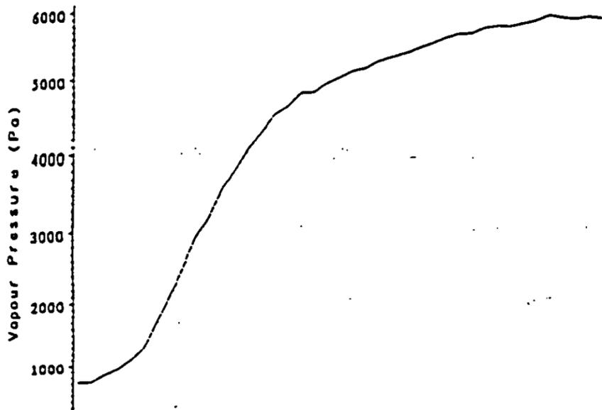
Figure 3 Typical vapor pressures developed under roof with simulated solar heating
