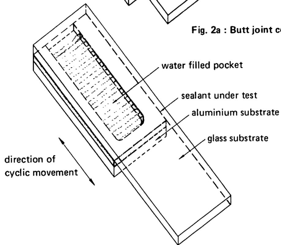
**Fig. 2b : Shear joint configuration**
