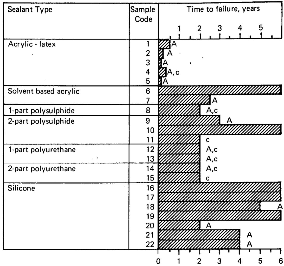
Fig 3 : Results for butt joints
