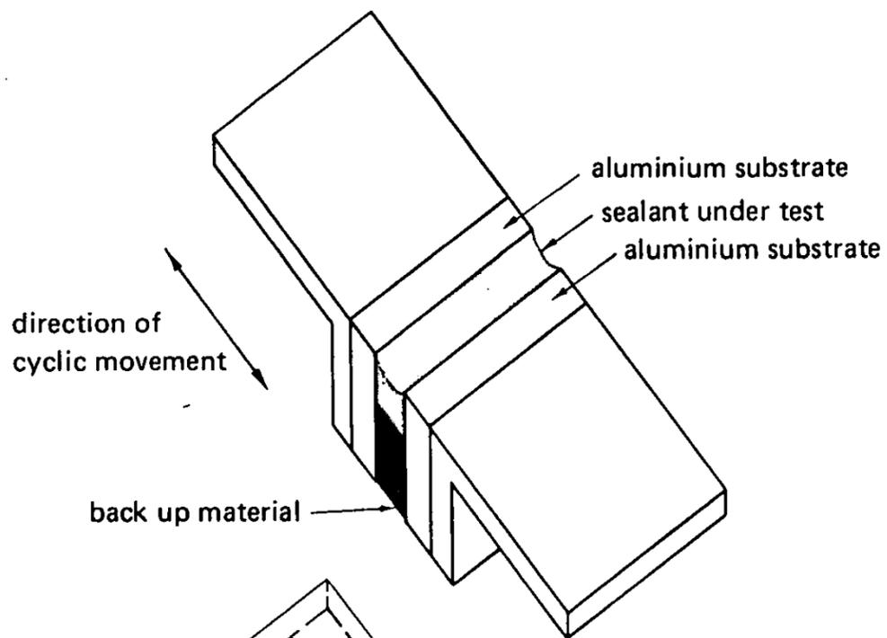
**Fig. 2a : Butt joint configuration**
