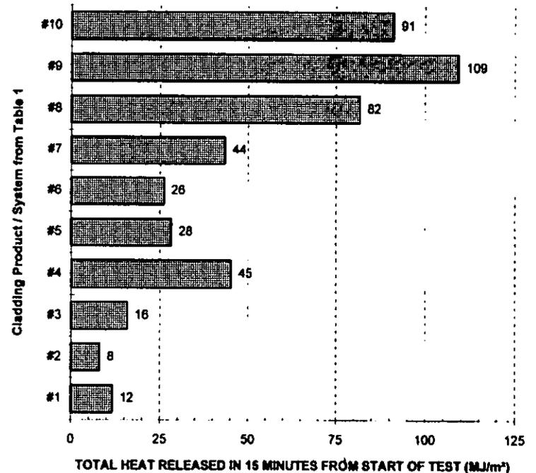
Figure 4. Total heat released in 15 min from start of test.
