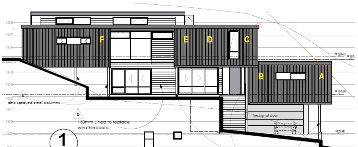
Figure 3. Elevation and location of TSC cladding.
