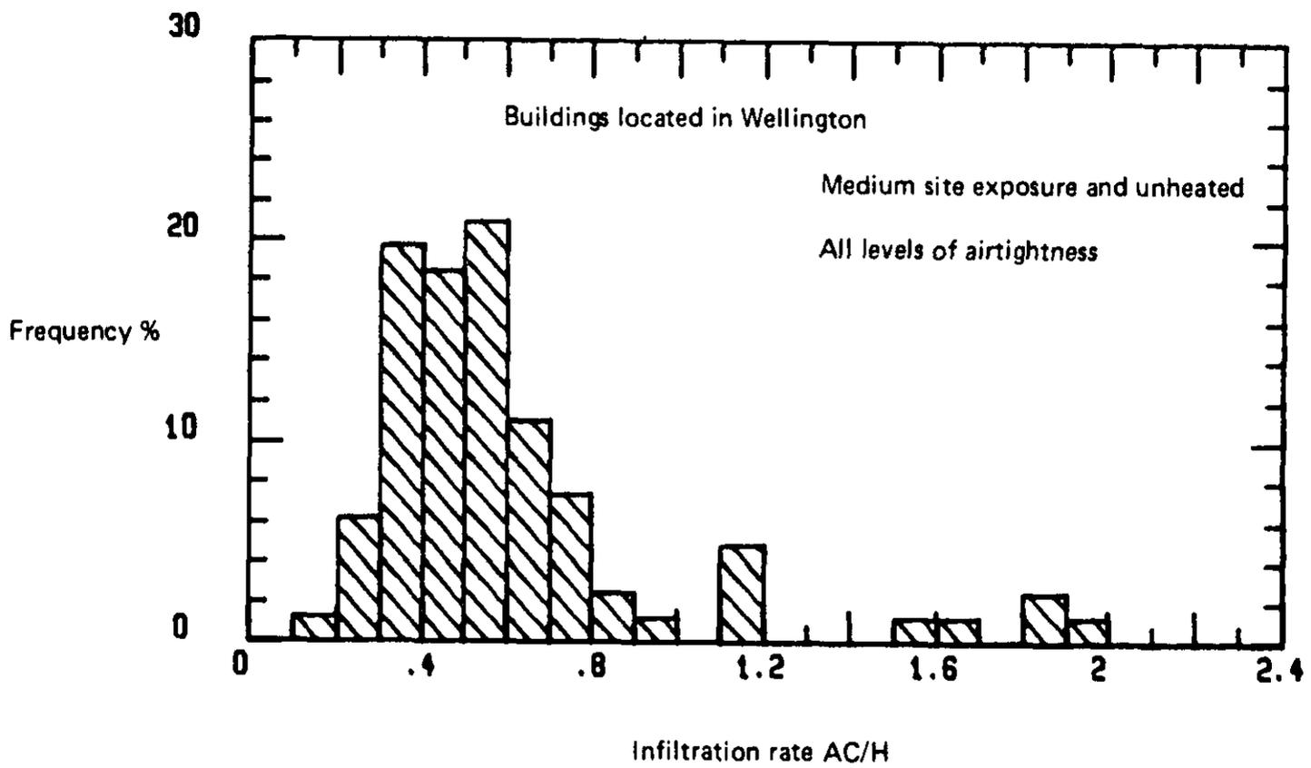
Fig 8 : Mean winter infiltration rate for buildings over the entire range of air tightness but with fixed wind exposure class.
