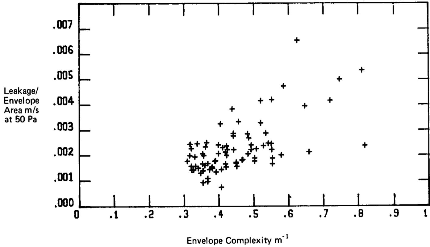
Fig 2: Measure of building envelope complexity against leakage/shell area at 50 Pa.
