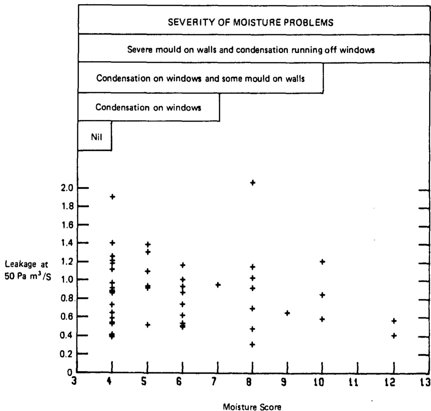
**Fig 11: Leakage rates at 50 Pa for houses in Christchurch and Auckland against moisture scores**
