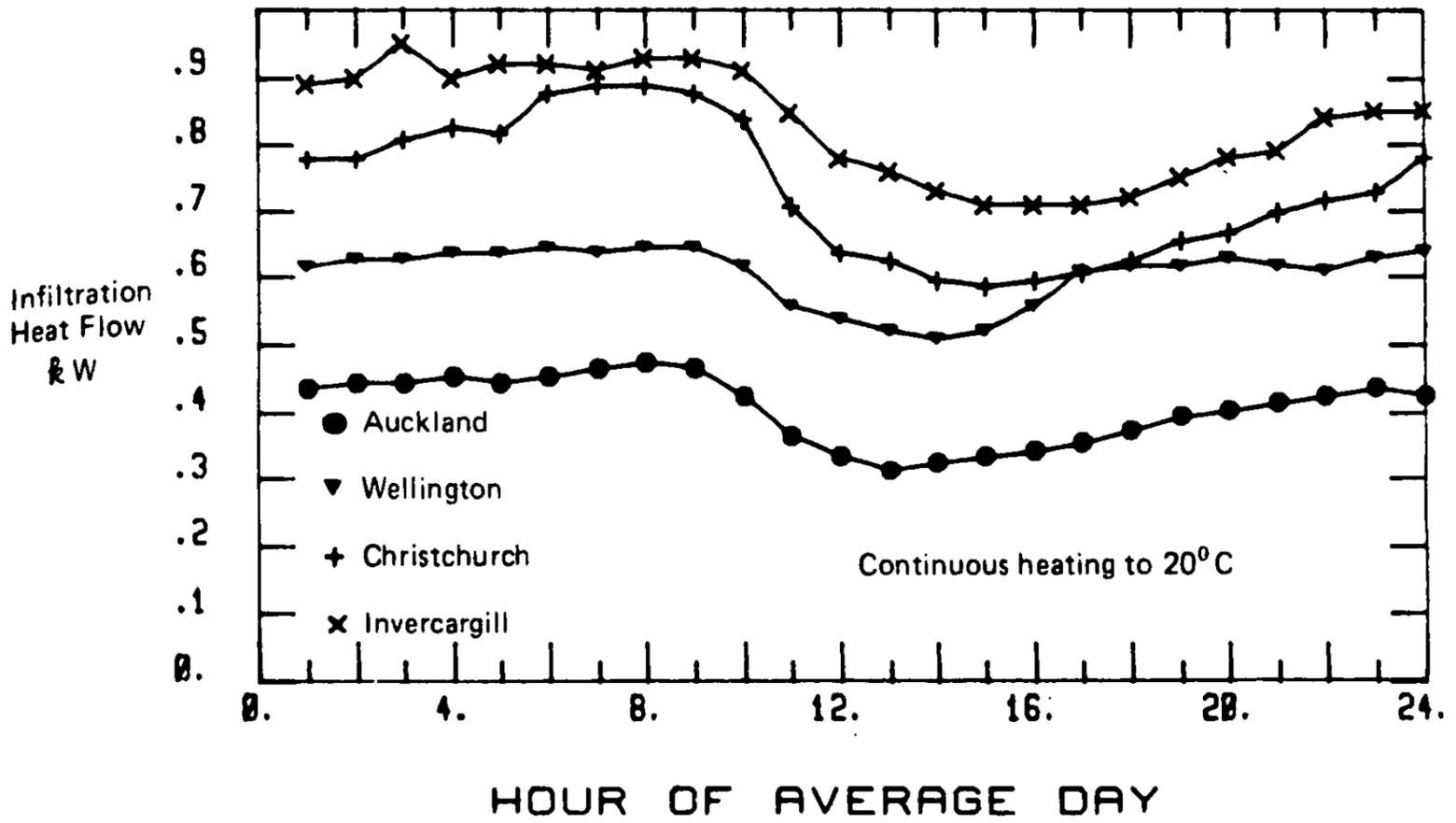
Fig 9: Winter average infiltration heat loss for a reference building sited with medium wind exposure and heated continuously to 20°C
