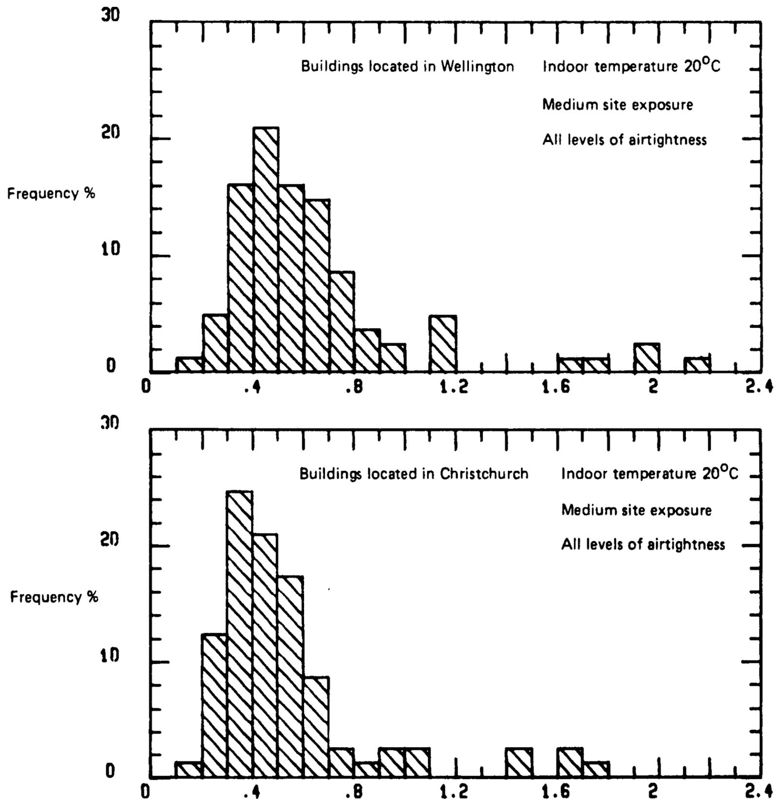
Fig 6 and 7 : Mean winter infiltration rates for buildings over the entire range of air tightness but with fixed wind exposure class.
