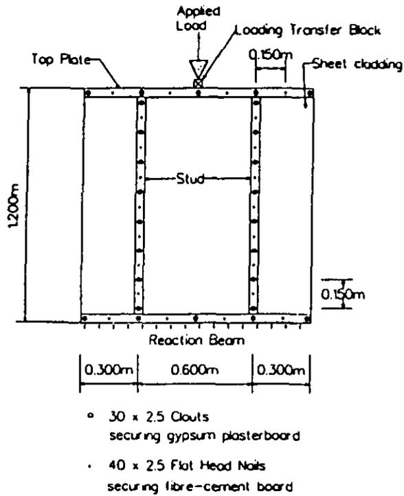
Figure 4 Elevation of top plate test specimen
