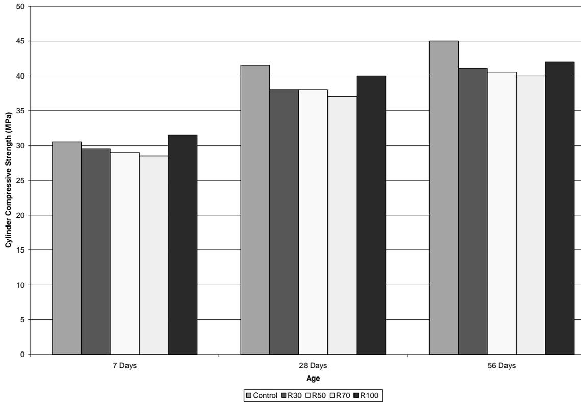
**Figure 6 Second Laboratory Trial Compressive Strengths**
