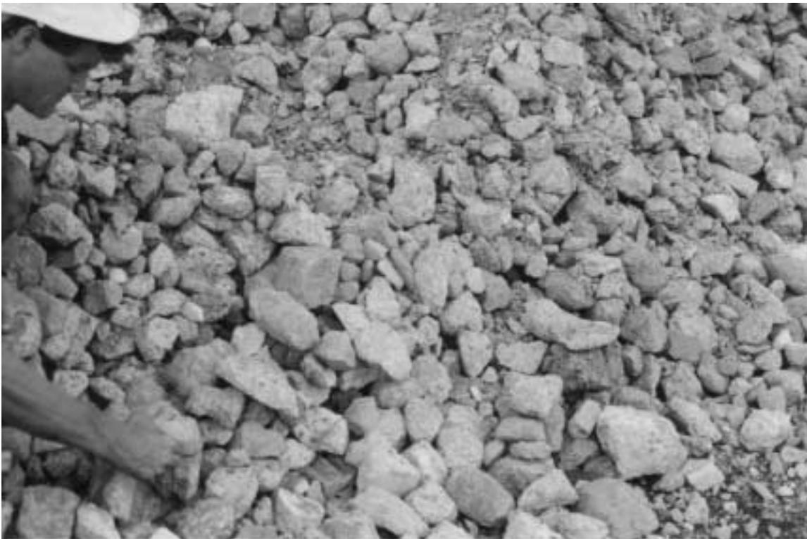
**Figure 2 Demolition Rubble After Processing**
