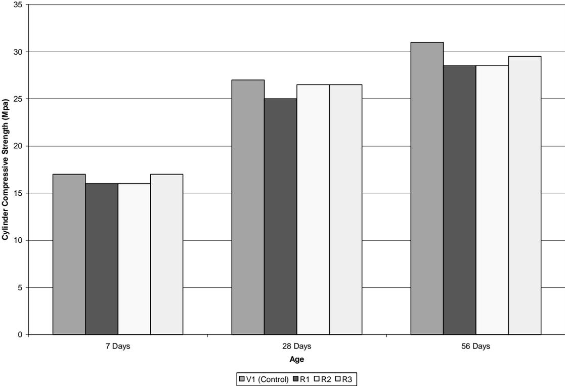
**Figure 4 First Laboratory Trial Compressive Strengths**
