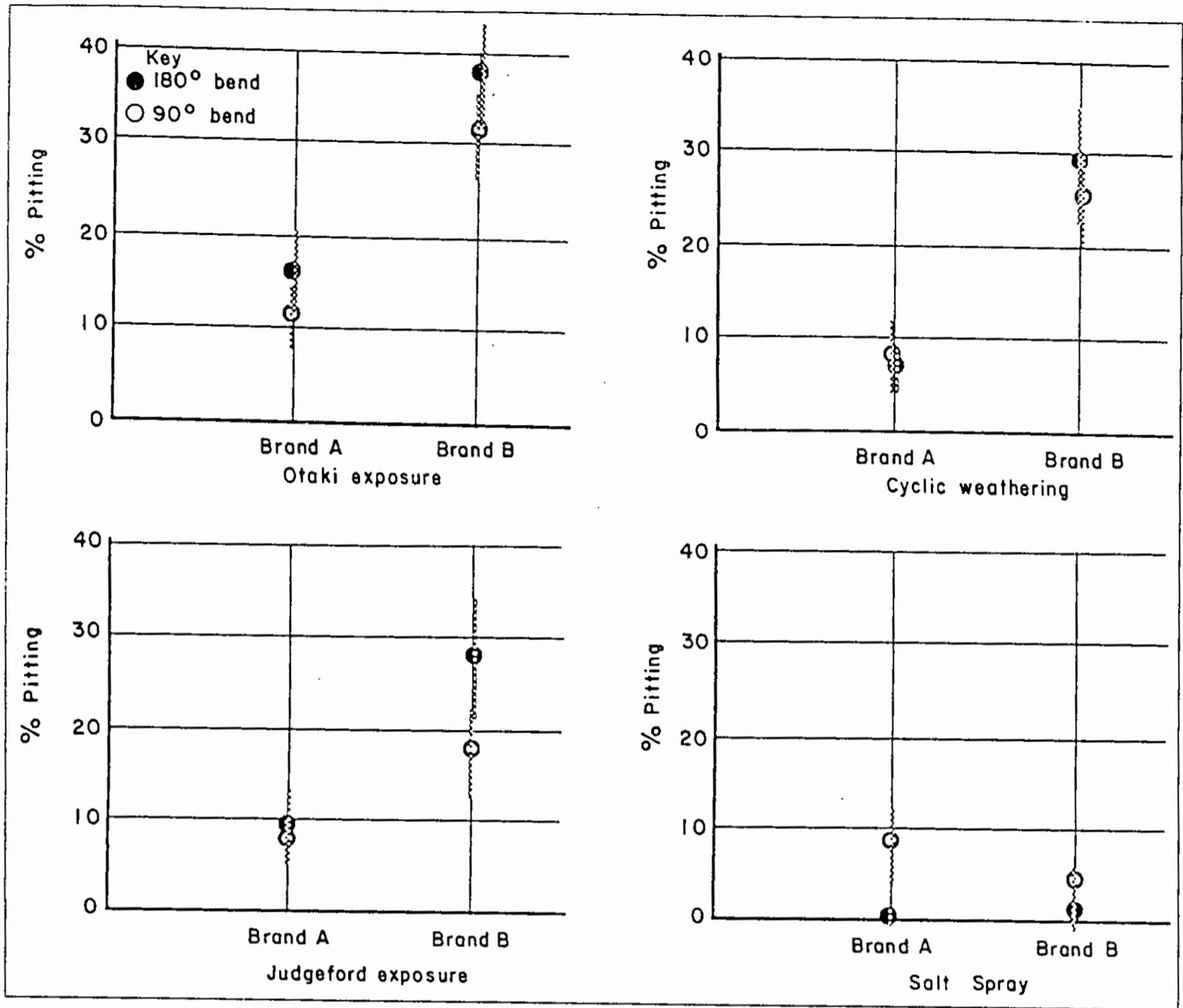
Fig 3 Pitting results for each exposure
