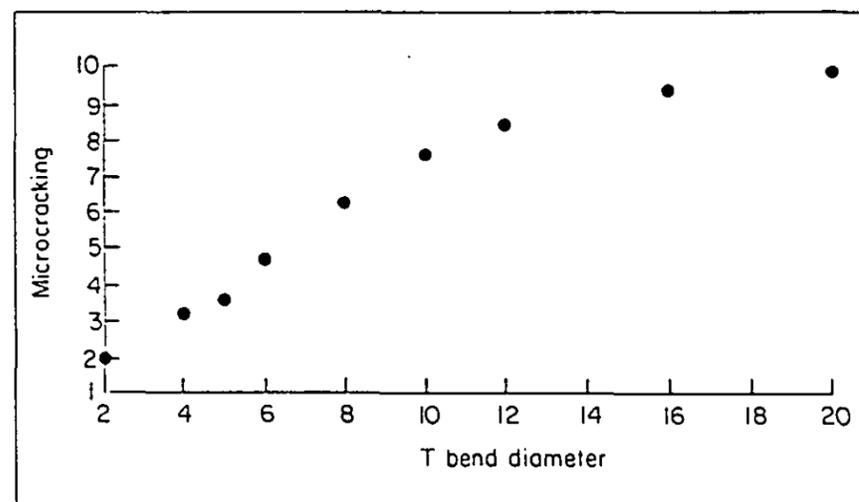
Fig 2 Microcracking for each T bend diameter
