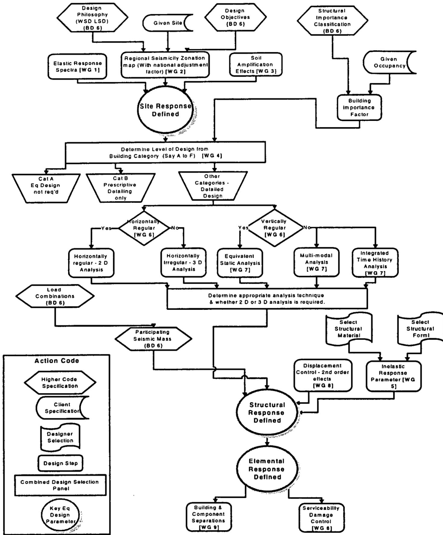
Proposed Structure for a Common Earthquake Design Standard
