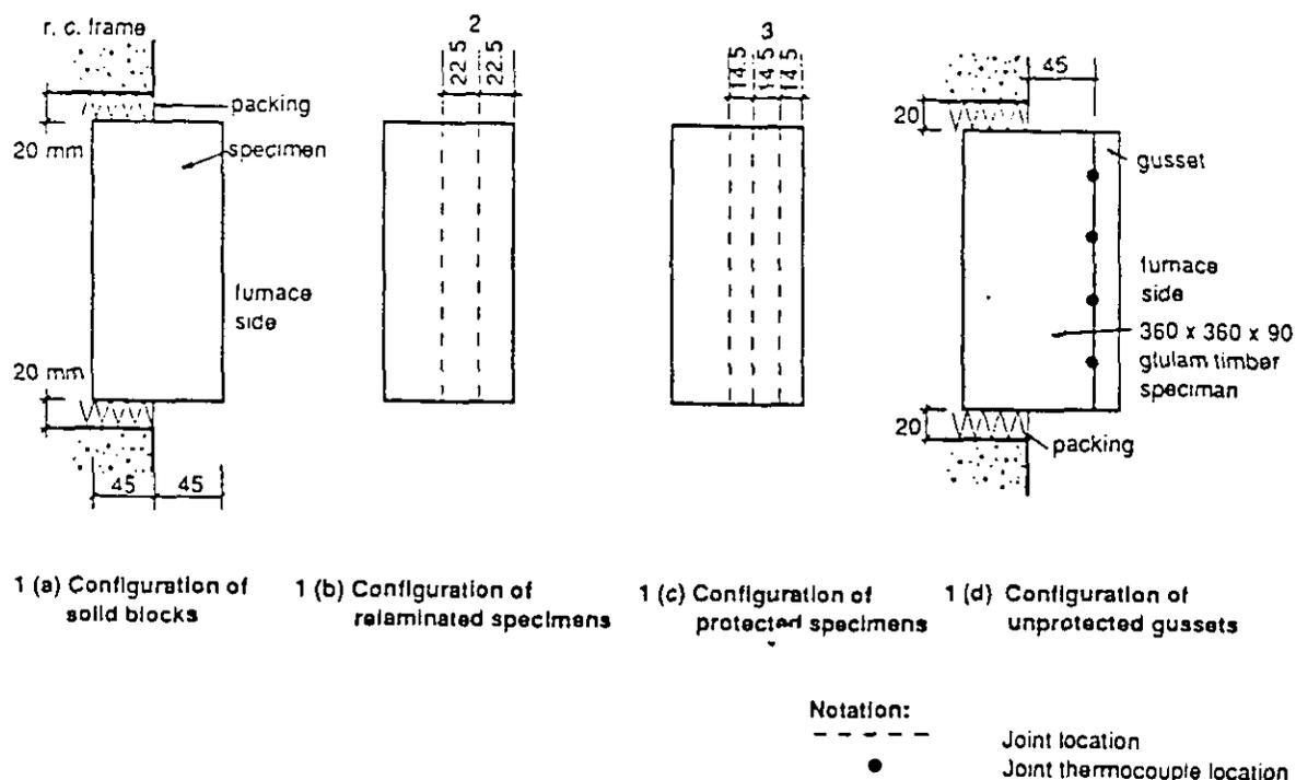
Figure 1 : Block specimen details
