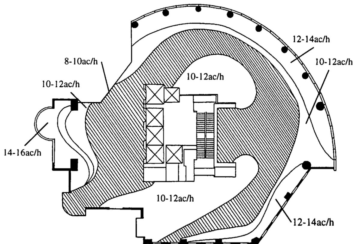
Figure 4: Approximate contours of effective ventilation rate in the breathing zones of building F.
