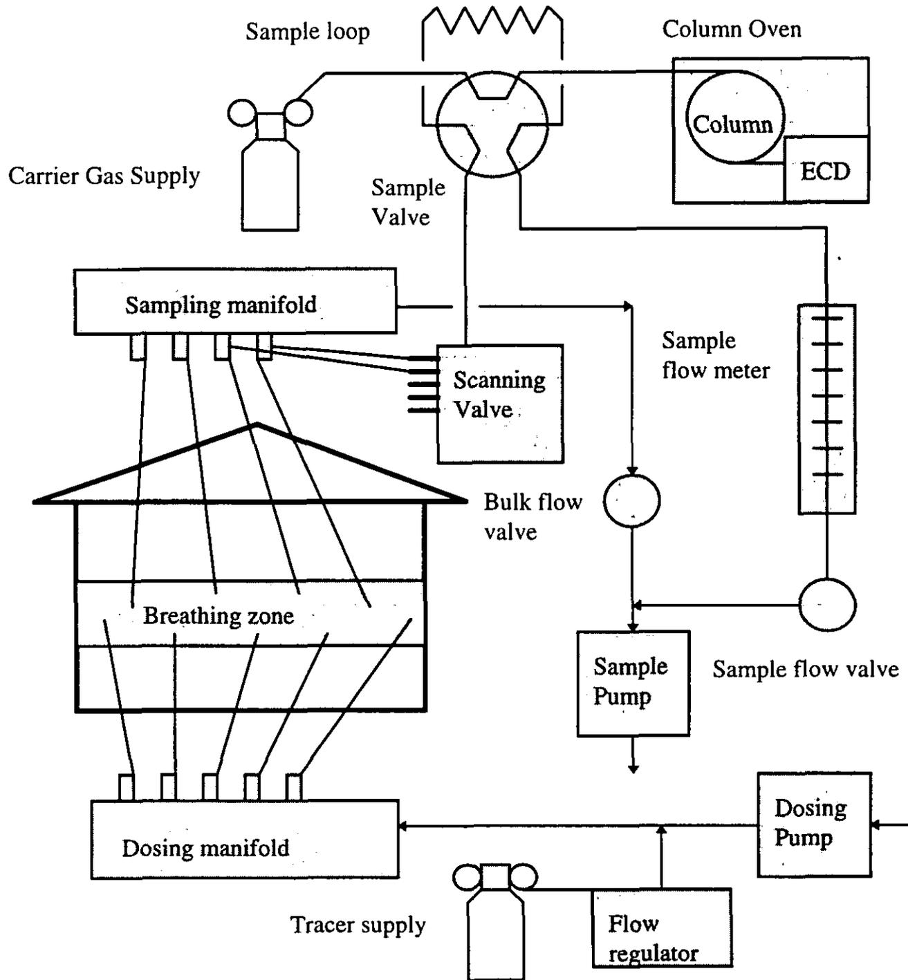
Figure 1: Outline of tracer dosing and sampling equipment for measuring ventilation performance.
