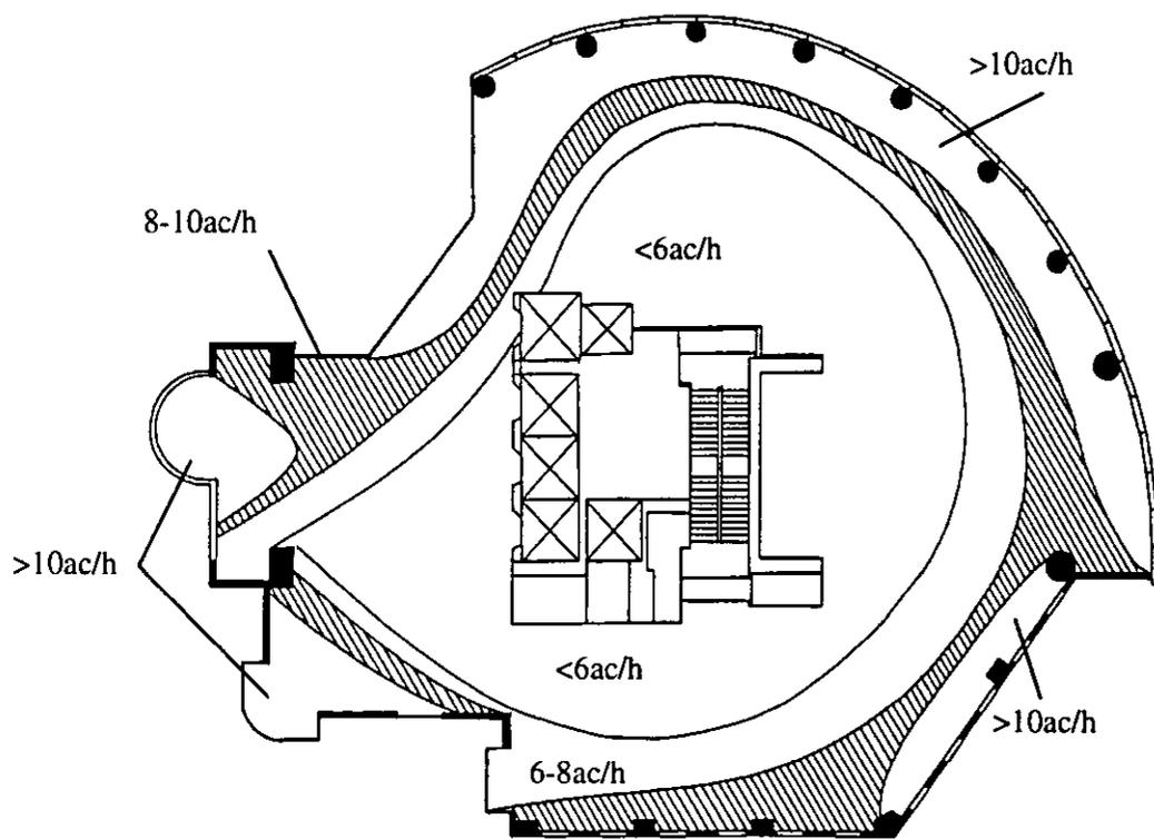
Figure 5: Approximate contours of air flow discharged through the ceiling in building F.
