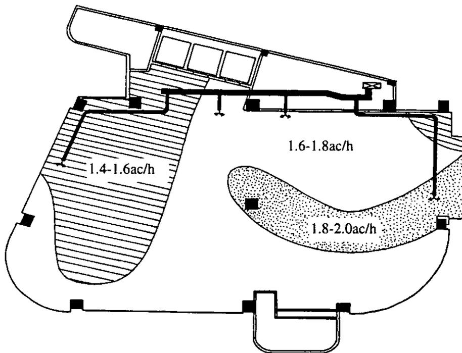
Figure 6: Approximate contours of effective ventilation rate in the breathing zones of building G.
