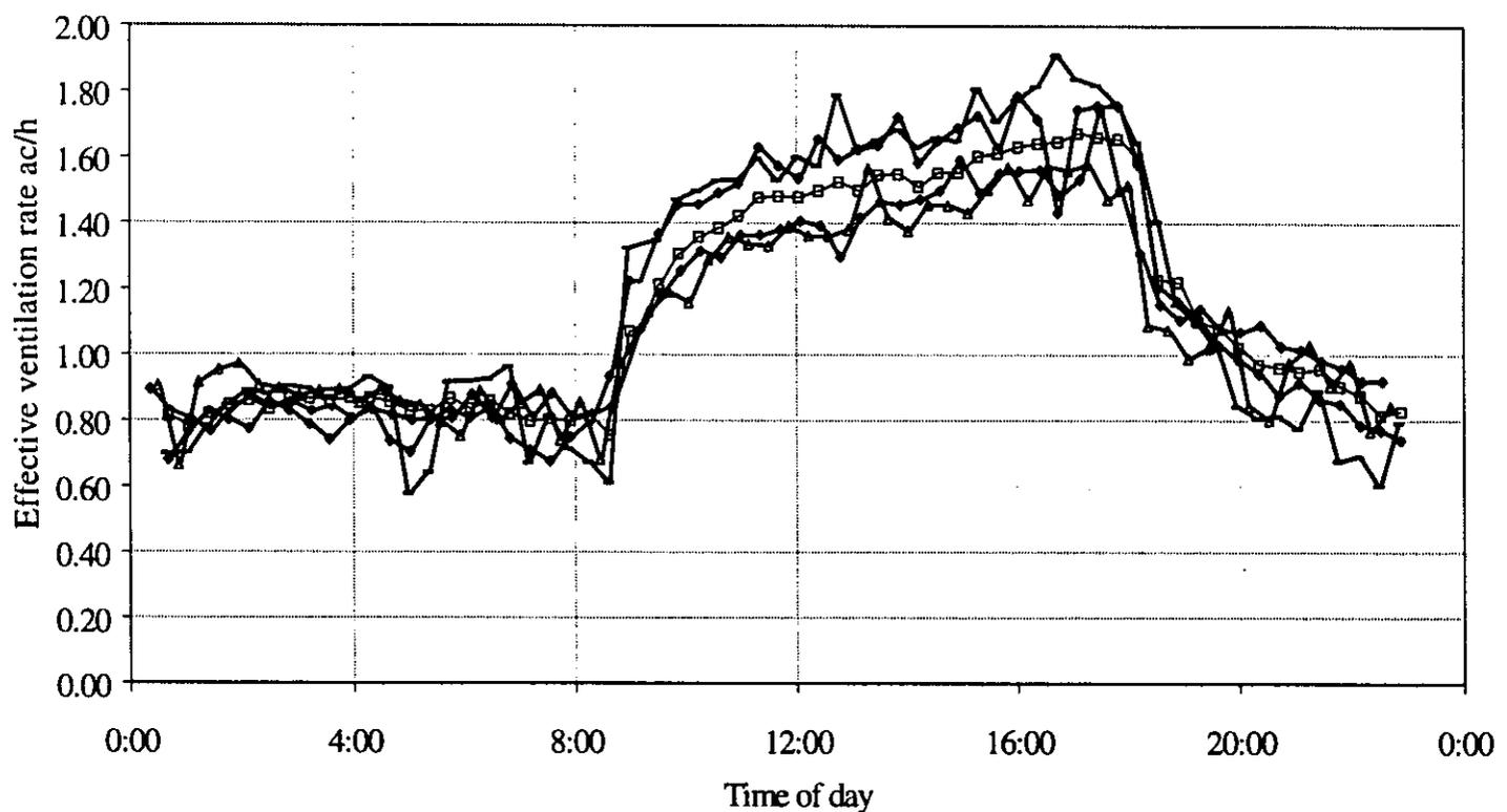
Figure 3: Effective ventilation rates in the breathing zones of building G.
