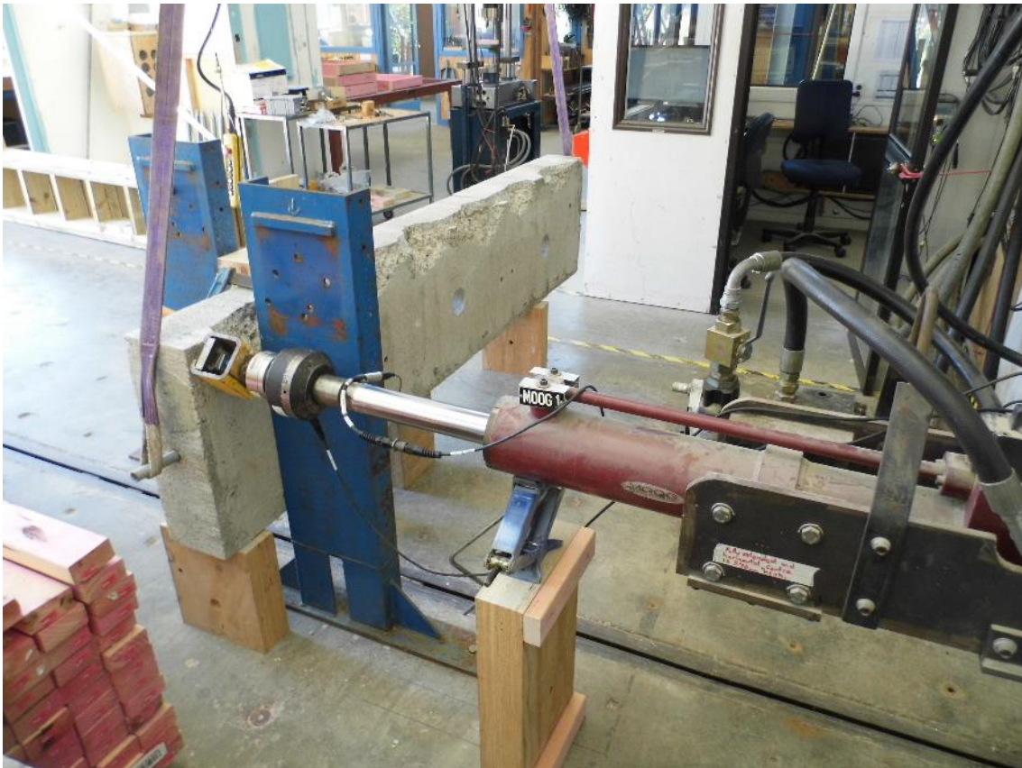
Figure 7. View of the test set-up for the anchor testing.
