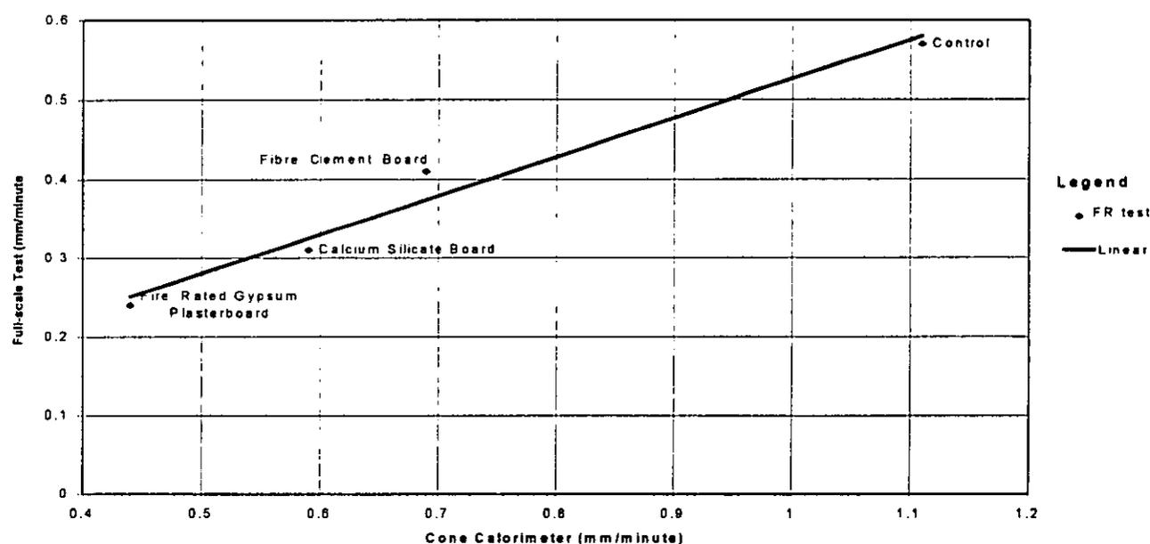
Figure 9. Correlation between the effective charring rates determined from the cone calorimeter and the full-scale tests.
