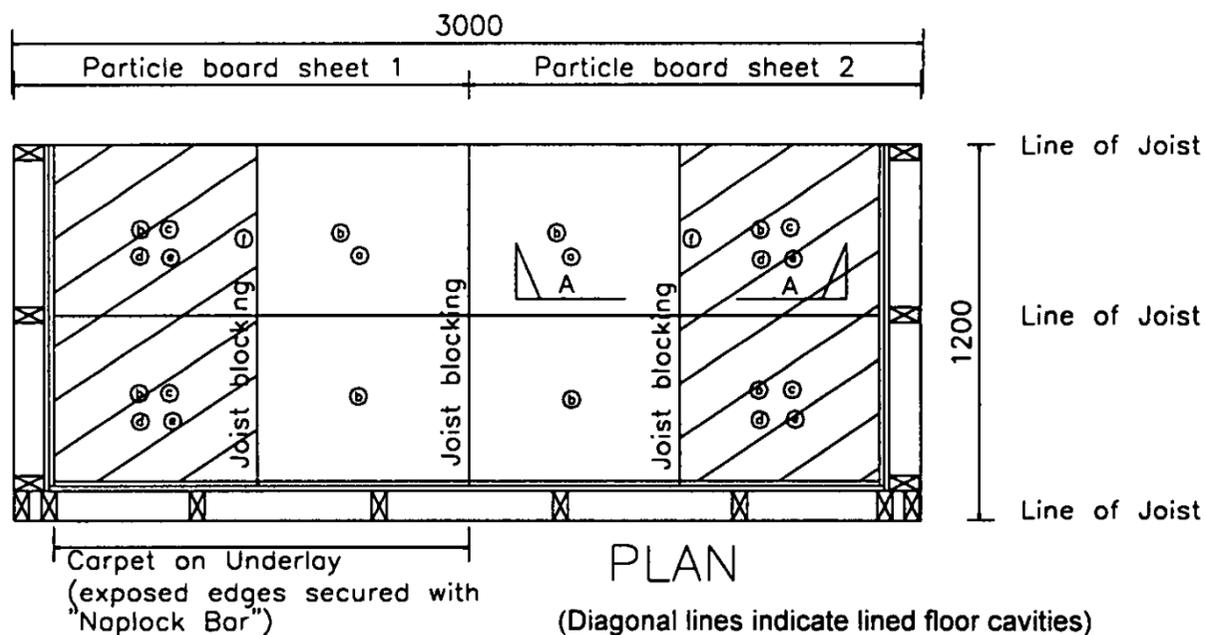
Figure 3. Floor plan for full-scale fire test 1.
