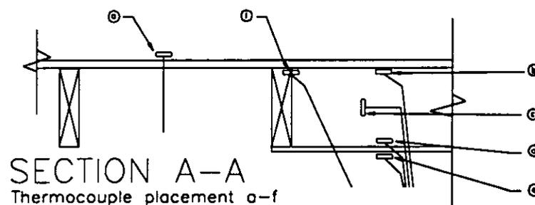
Figure 4. Floor section identifying location of thermocouples, full-scale test 1.
