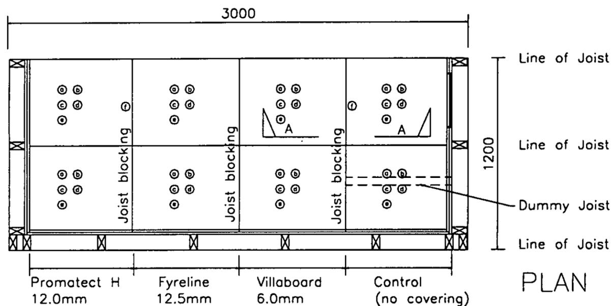
Figure 5. Floor plan for full-scale test 2.
