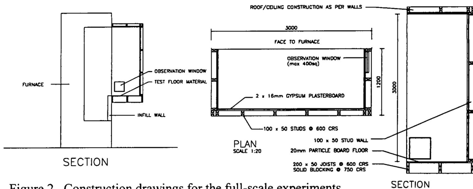
Figure 2. Construction drawings for the full-scale experiments.
