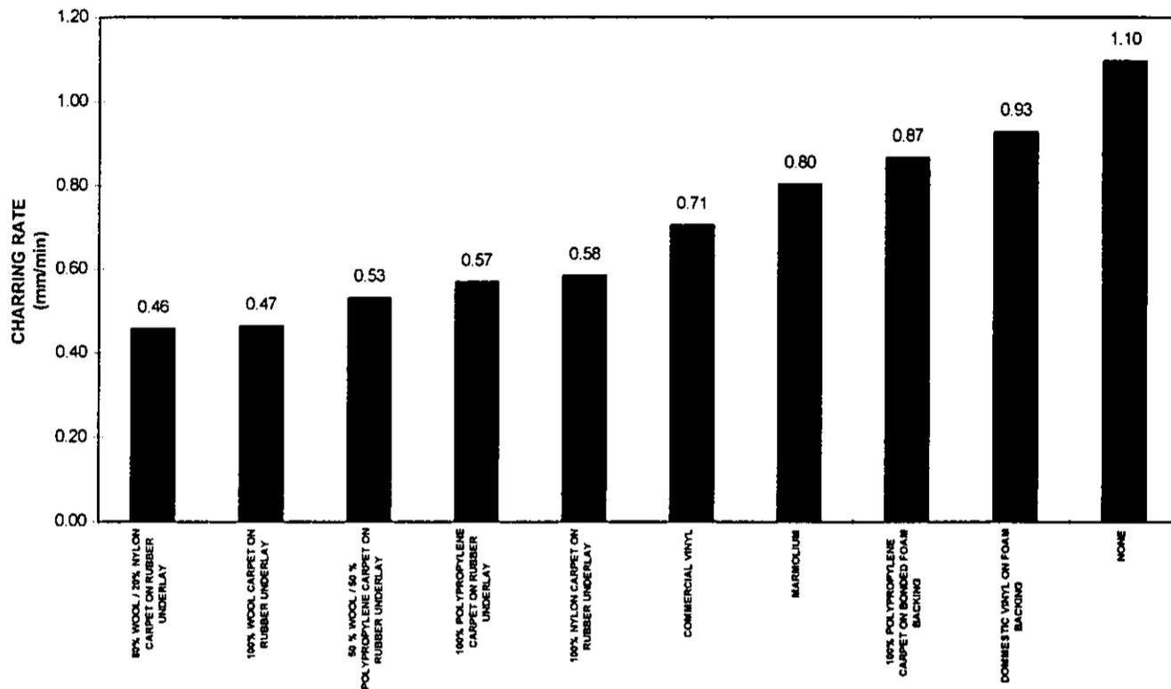
Figure 1. The effective charring rate of the particleboard under various floor coverings, measured in a cone calorimeter at 75 kW/m<sup>2</sup>.
