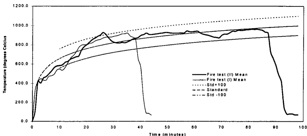
Figure 7. Furnace time temperature curves fire tests 1 and 2.
