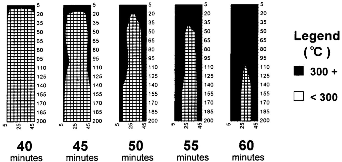
Figure 8. Charring front profile over time for the dummy joist.
