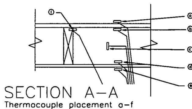
Figure 6. Floor section identifying location of thermocouples, full-scale test 2.
