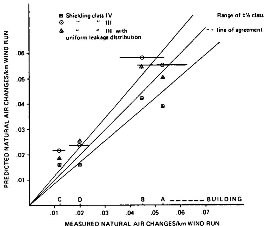
FIG. 7—Correlation of infiltration rate predictions using LBL model with experiment.
