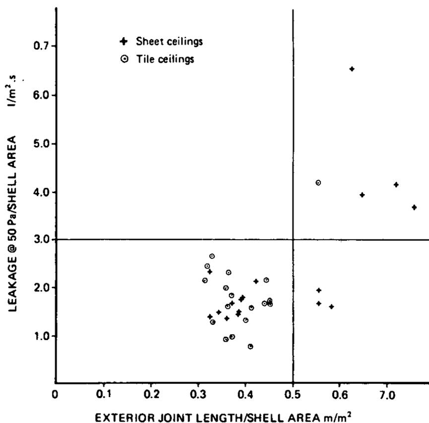
FIG. 4—Measure of building shell complexity against leakage/shell area at 50 Pa.
