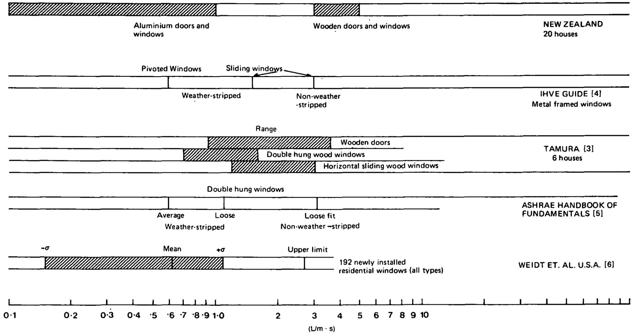
FIG. 5—Results of window/door leakage tests.
