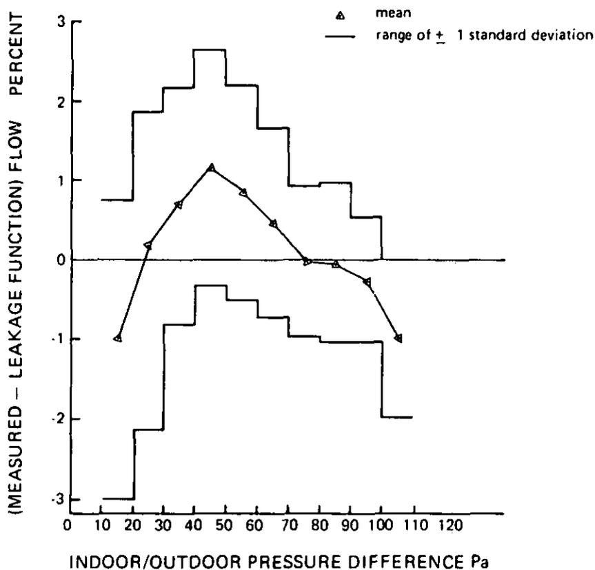
FIG. 2—Correlation of residuals with pressure. Mean and standard deviation for 50 airtightness tests.
