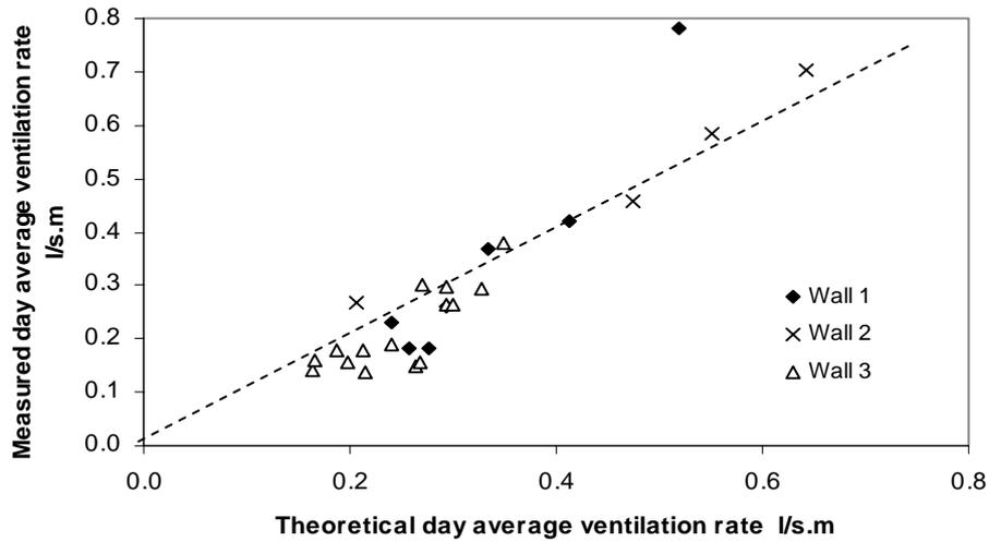
**Figure 4: Day average ventilation rates in open rainscreen wall cavities.**
