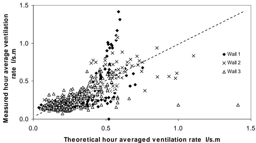
**Figure 5: Hour averaged ventilation rates in open rainscreen wall cavities.**
