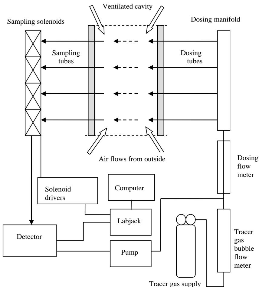
**Figure 1: Configuration of tracer based equipment for measuring cavity ventilation rates.**
