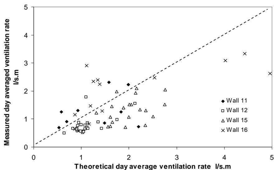
**Figure 6: Day averaged ventilation rates in drained and ventilated wall cavities with line of agreement.**
