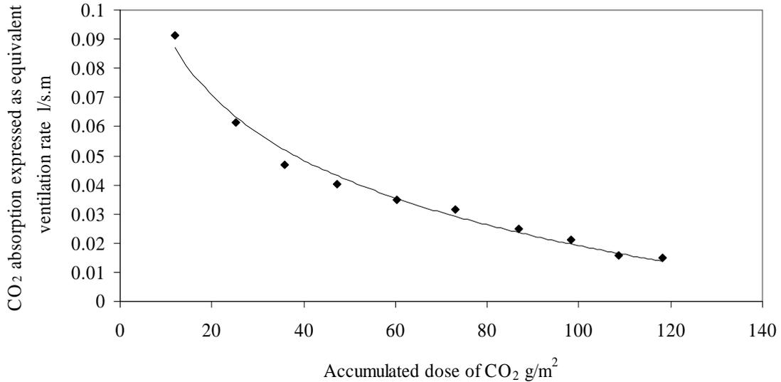
**Figure 2: Absorption of CO<sub>2</sub> in fibre cement materials declining as the carbonation processes advances.**
