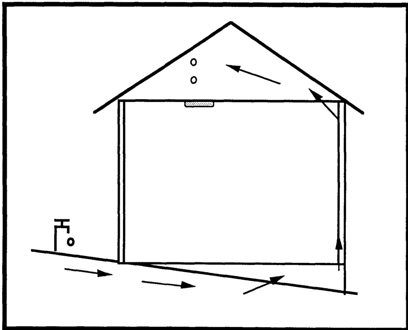
**Figure 4:** One of the more interesting causal sequences embodied in the DAMP system. Ground water from a leaking tap travels under a house where it evaporates. The stucco wall construction provides a convenient path for sun aided convection to transport the moist air to the roof space. In the evening the moist air condenses on the cold roof. Water then drips onto the ceiling, causing a stain.
