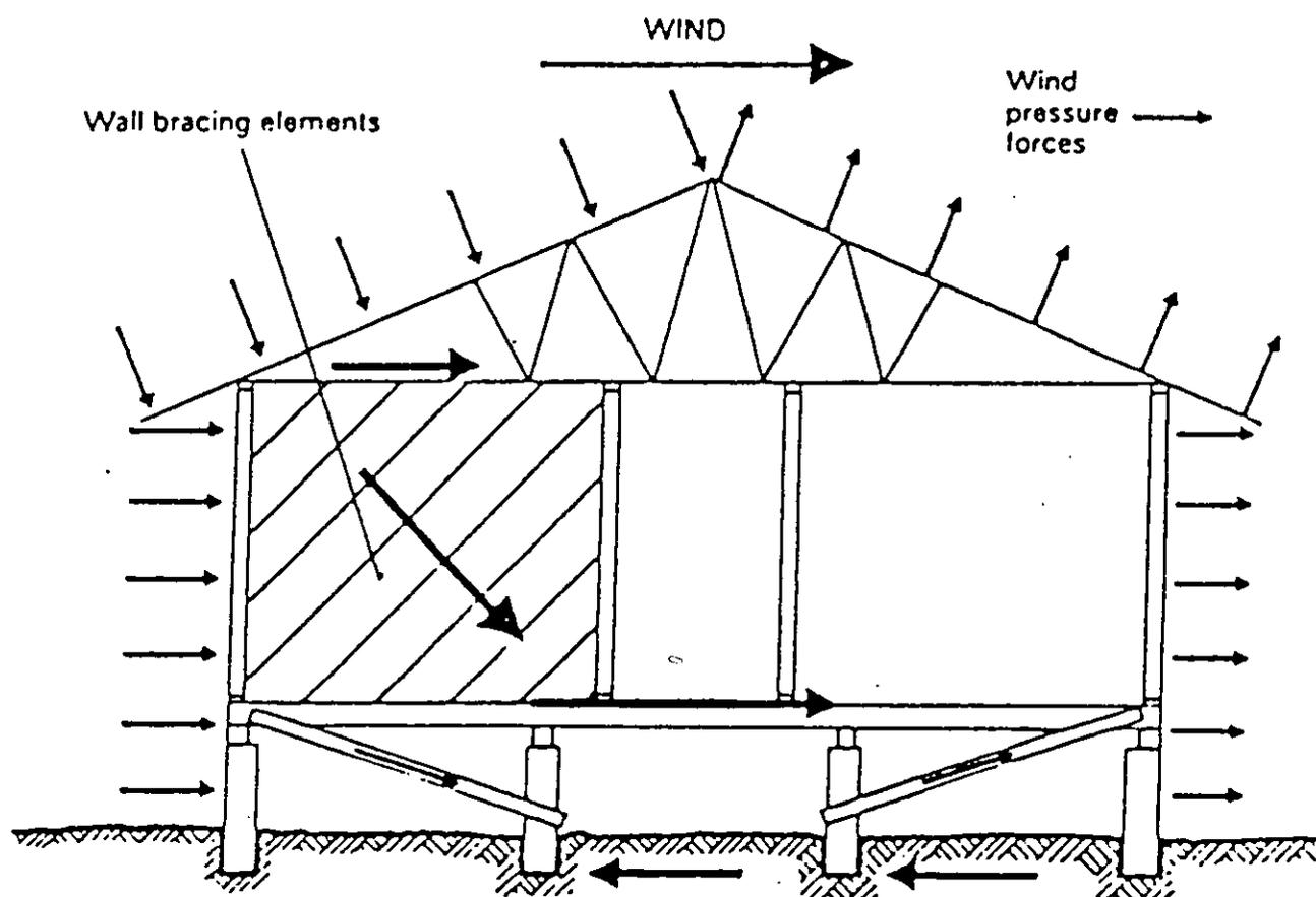
Figure 3: Action of Wind Forces on a Building
