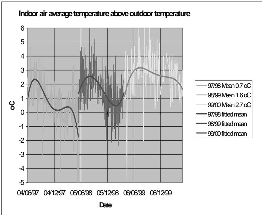
**Figure 2: Daily Average House Temperature in Excess of Outdoor Temperature**
