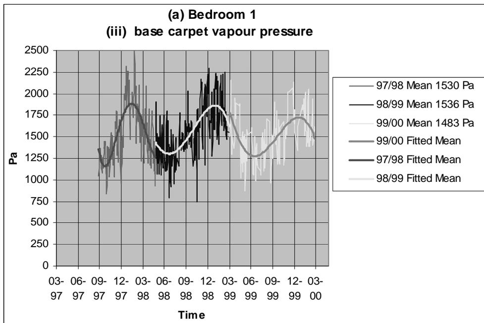
**Figure 8: Base of carpet vapour pressures**
