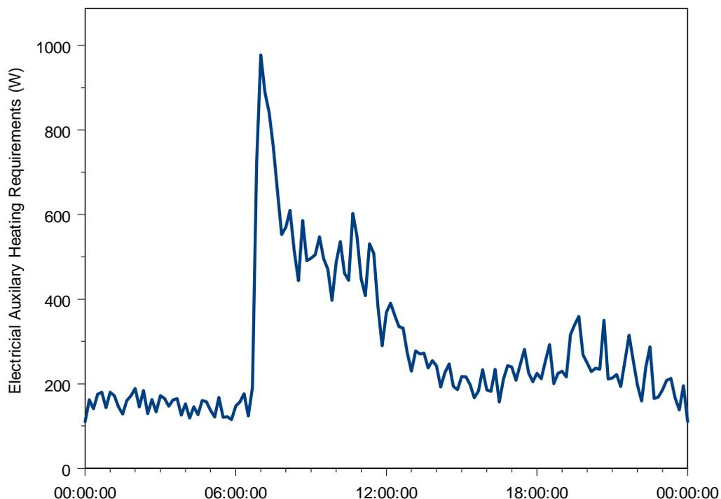
**Figure 1. The daily electrical supplemental heating from one of the SWH monitored houses.**
