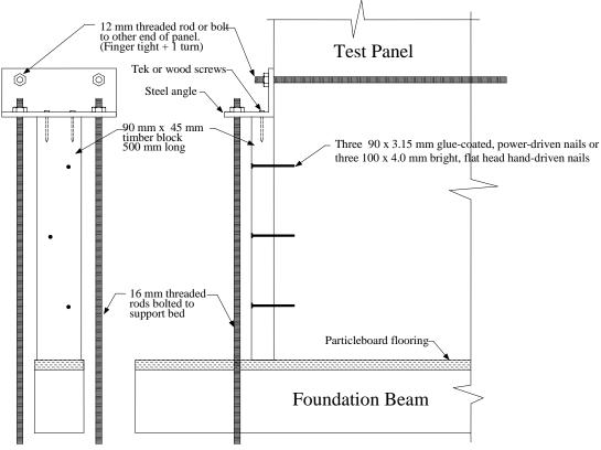
Figure 2. Supplementary uplift restraint
