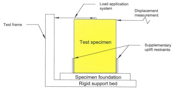
Figure 1. Test arrangement
