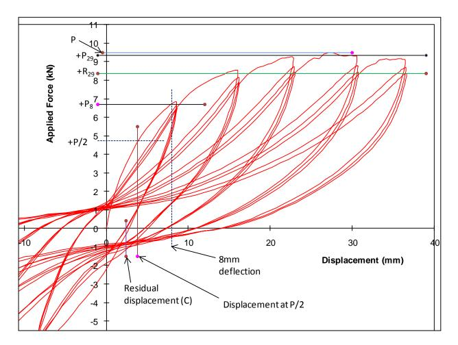
Figure 4. Force and displacement measurements (for y = 29mm)
