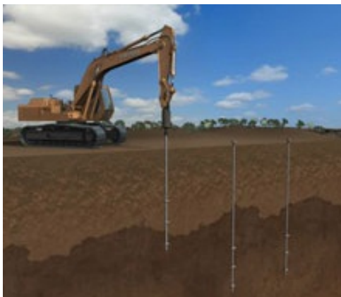
Figure 14: Helical pier piles are screwed through the ground into a stable substrate (Basement Systems, 2012). Figure 15: Precast concrete piles are driven into the ground (Simplex Westpile, 2012).
