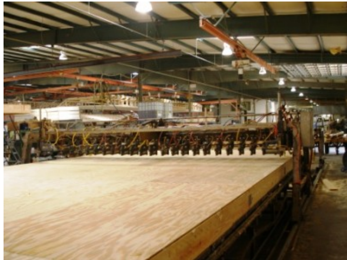
Figure 5: An automated production line processes timber panels (Oasis Homes, 2012).
