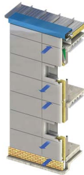
Figure 9: Rainscreens allow water to exit and air to dry the cavity (Euroclad, 2012).
