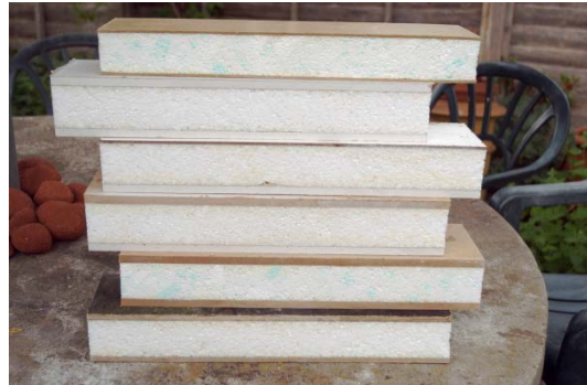
Figure 31: SIPs come in a number of material combinations. Image: Ashley Balsam Baz (Rodriguez, 2013).
