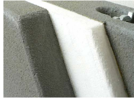
Figure 29: Insulated concrete sandwich panel (Reid Construction, 2012).
