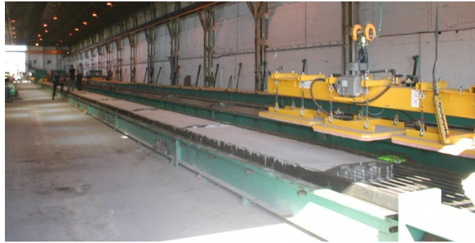
Figure 26: Precast concrete panels can be pre-tensioned to minimise panel thickness, provide higher structural rigidity and strength in tension and prevent slump (ACP Concrete Ltd, 2012).
