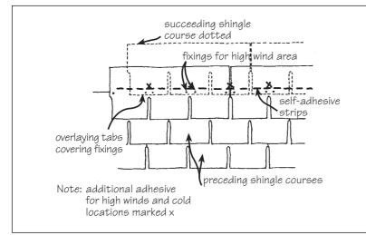
Figure 4. Shingle fixings.
