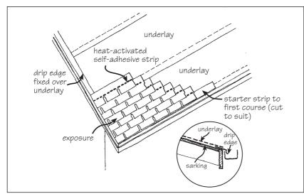
Figure 1: Standard underlay and shingle layout showing offsets.
