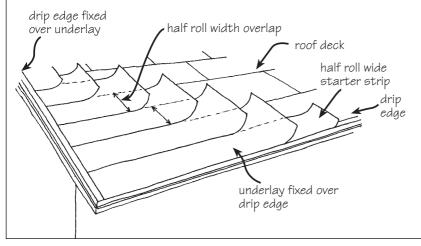
Figure 2. Underlay to low pitched roof.
