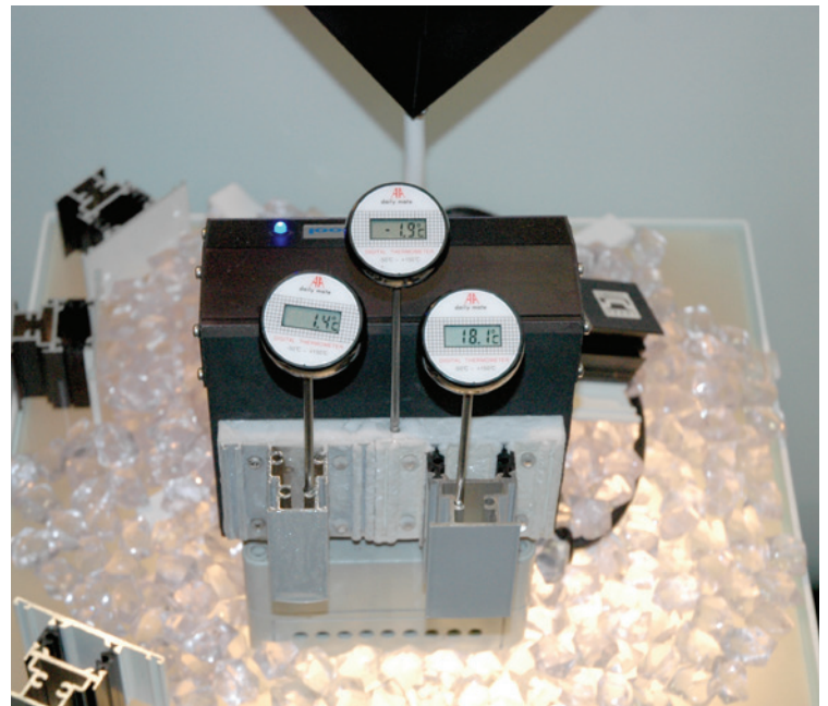
Figure 2: Display showing benefits of a thermally broken window
