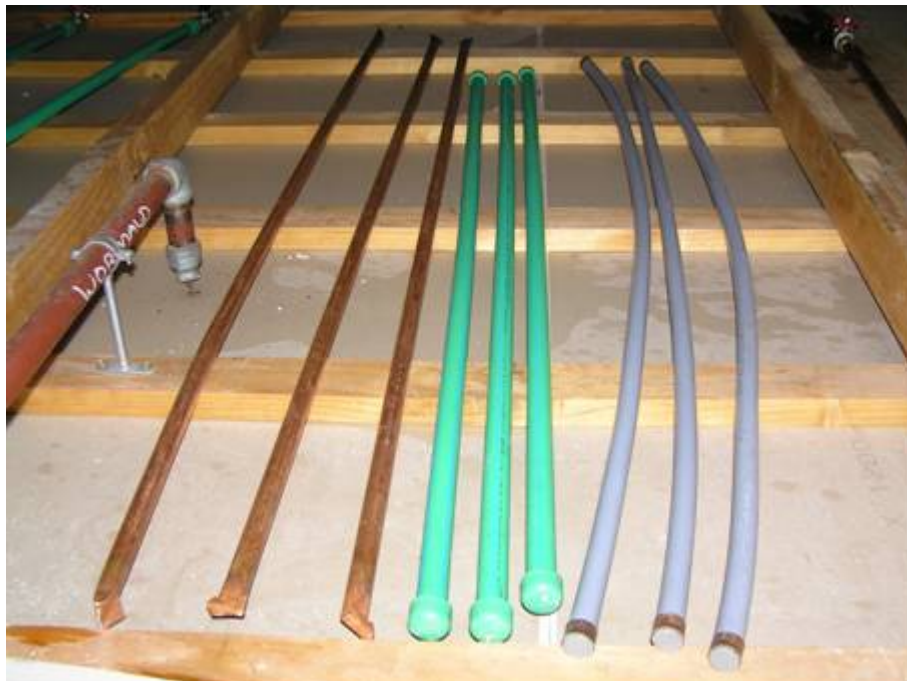
Figure 9: Pipes used for static water quality tests.
