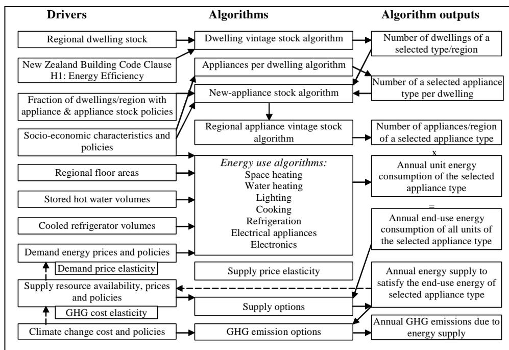
**Fig iii: 'Household Energy Efficiency Resource Assessment' (HEERA) flow diagram**
