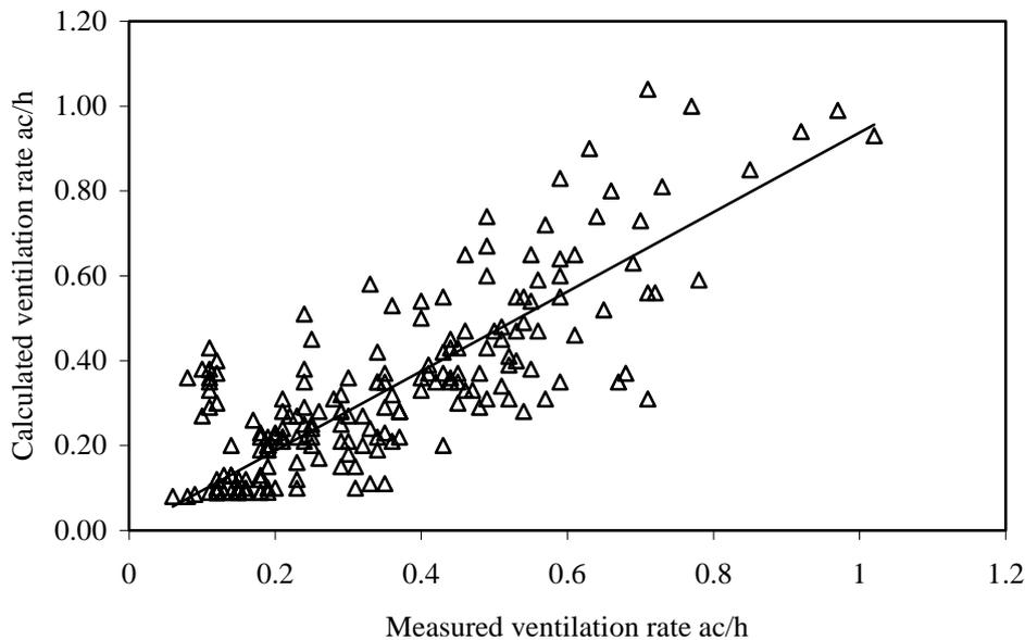
**Figure 2: Measured and calculated infiltration rates over half-hour periods for buildings A to F.**
