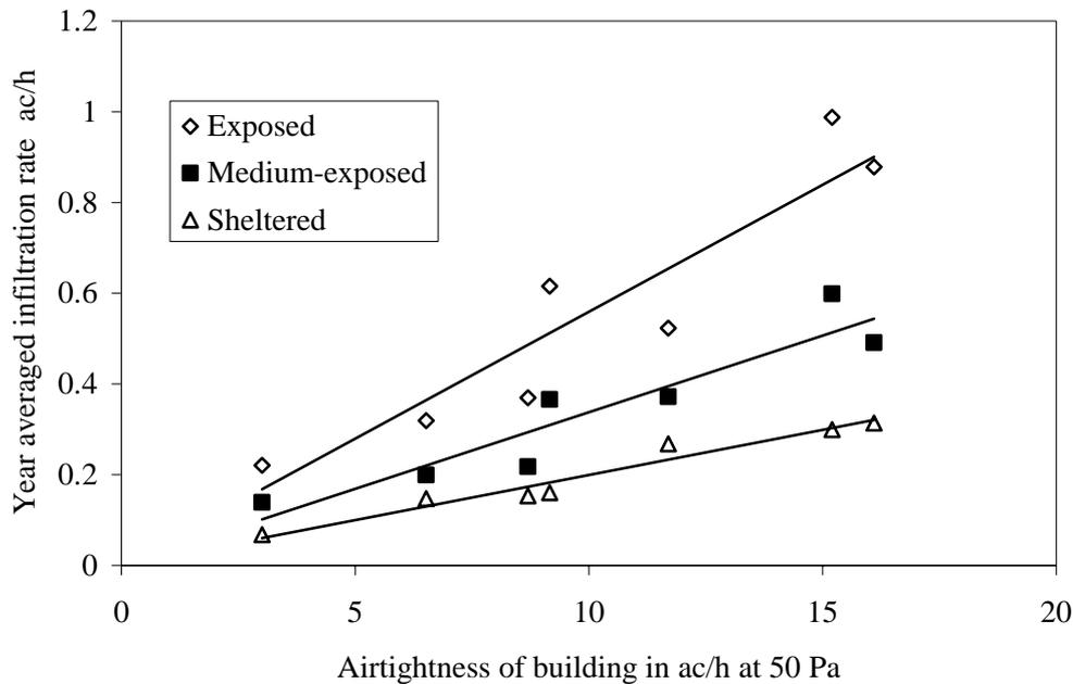
Figure 3: Climate averaged infiltration rates calculated using the BREEZE model for buildings with suspended floors with three wind exposure classifications.
