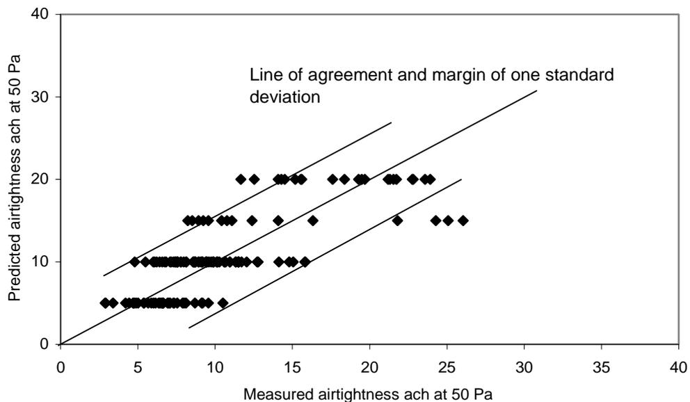
**Figure 1: Building airtightness measurements compared with airtightness classifications.**
