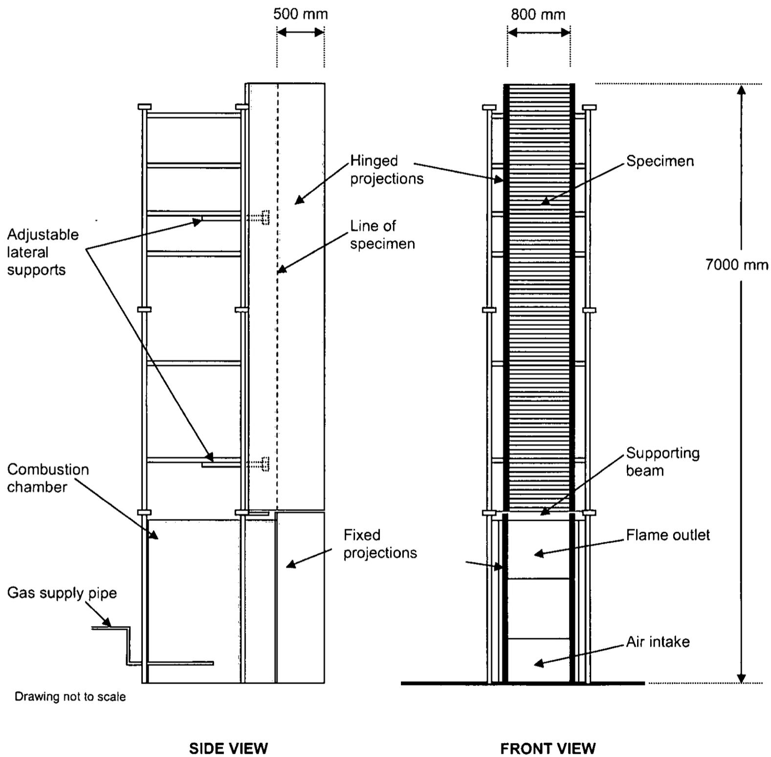
Figure 1. Test apparatus
