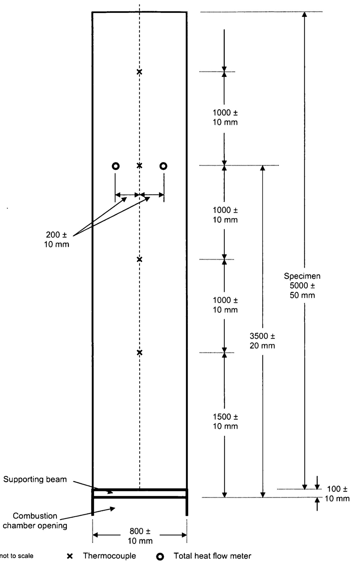
Figure 4. Specimen dimensions and instrumentation layout
