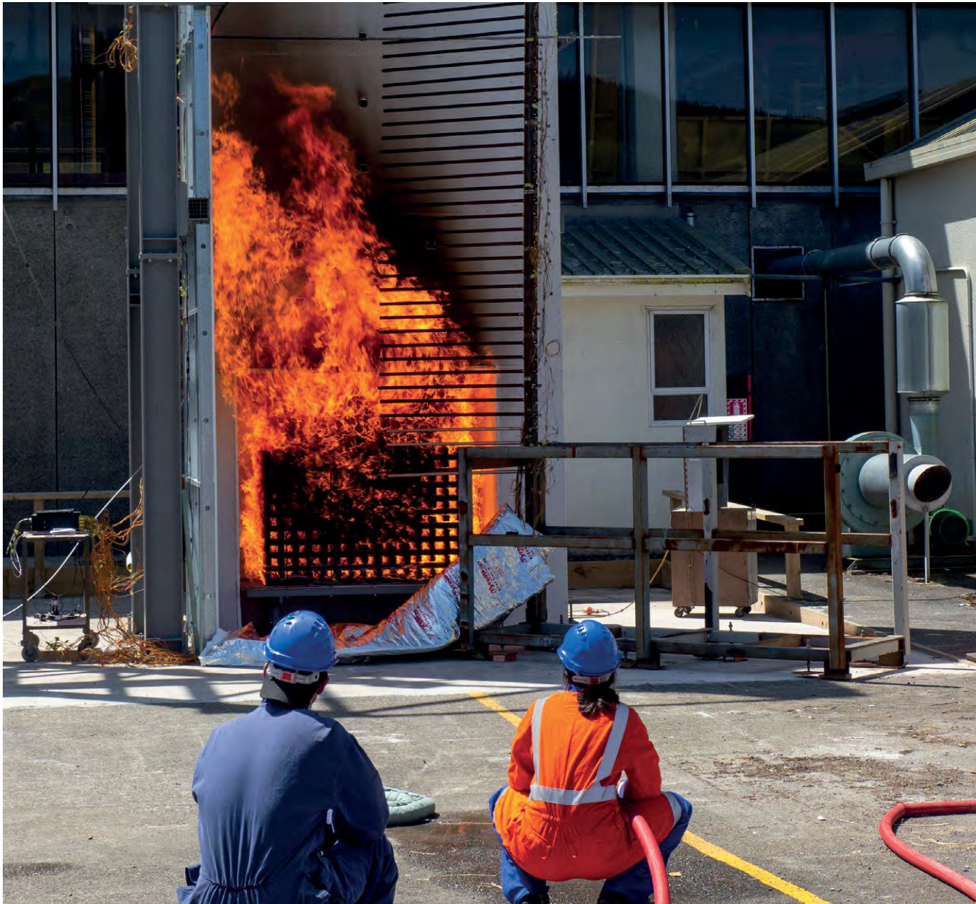
BRANZ's latest facility makes it possible to fire test full-scale façade systems.
