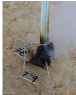
(c) Unexposed post-test
